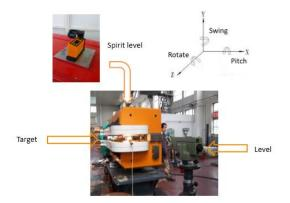
Fig.5 Adjusting the rotation of dipole by spirit level
