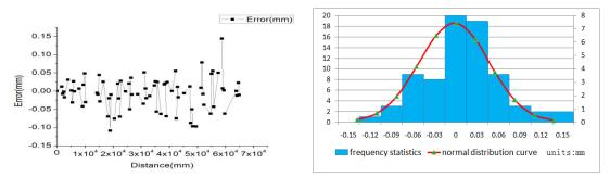
Fig.12 Y axis error distribution of mathematical statistical based on smoothing orbit
