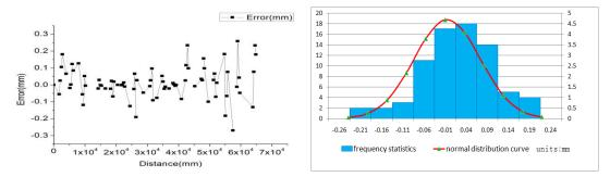
Fig.11 X axis error distribution of mathematical statistical based on smoothing orbit
