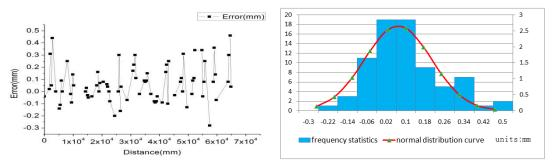
Fig.6 X axis error distribution of mathematical statistical based on theoretical orbit
