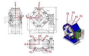
Fig.2 Internal reference marks and element coordinate system of each magnet The process of smoothing includes six steps as shown in Fig.3
