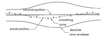
Fig.4 Position of magnets with respect to theoretical orbit
