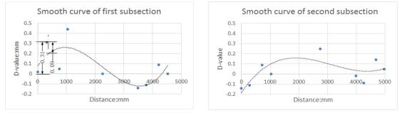
Fig.9 First subsection curve fitting
