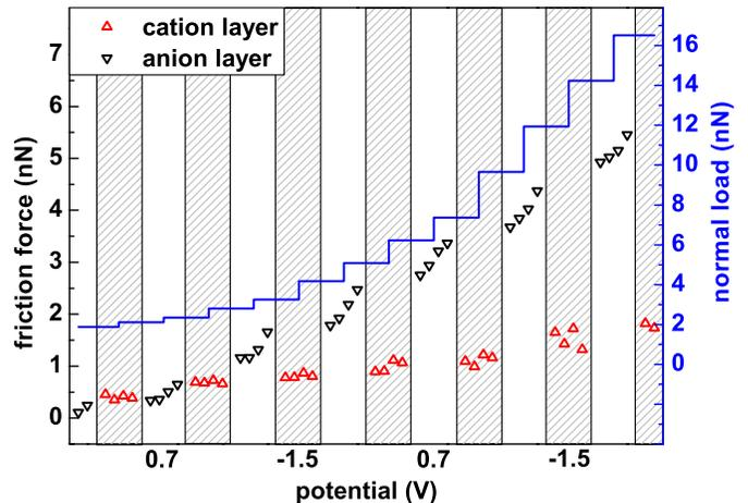
FIG. 4: Friction forces as functions of load and applied potential recorded for a sharp AFM tip sliding on Au(111) in [BMP<sup>+</sup>][FAP<sup>-</sup>]. Each data point represents the average over a full scan frame of 14 nm side length. The potential is switched between -1.5 and 0.7 V for each value of the applied normal load. Reprinted with permission from reference 52; Copyright 2012 by the American Physical Society.
