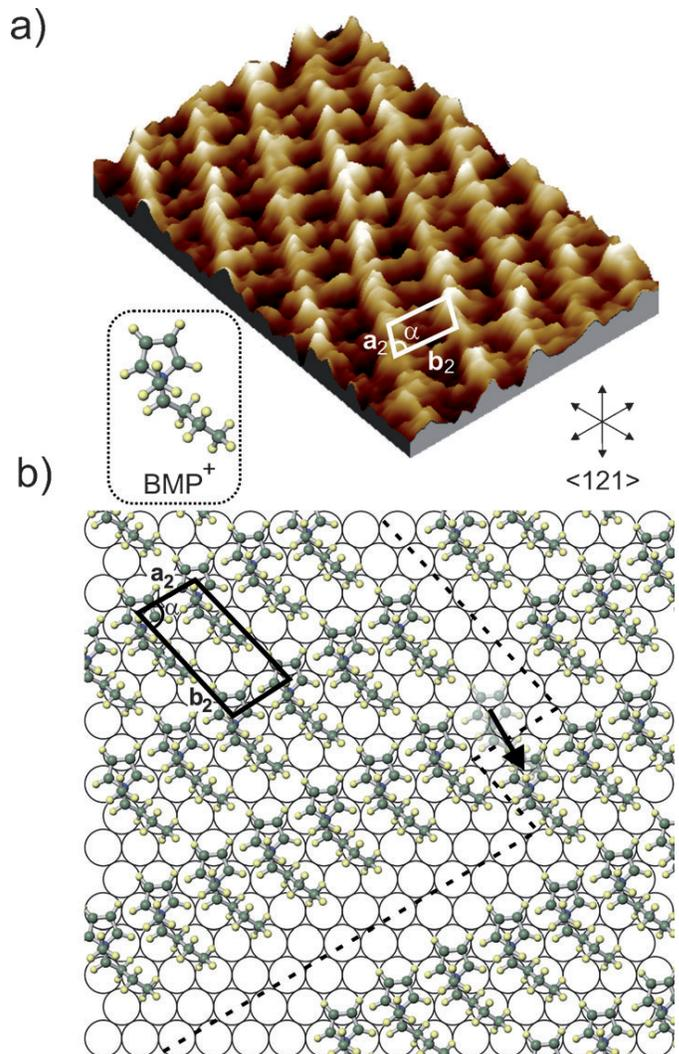
FIG. 1: a) High-resolution STM image ( $5.4 \text{ nm} \times 7.5 \text{ nm}$ ) of the  $\text{BMP}^+$  adlayer on Au(111) at  $-1.4$  V and b) proposed structural model, showing two domains of the  $(\sqrt{3} \times \sqrt{3})$   $\text{BMP}^+$  adlayer separated by a translational domain boundary (indicated by dashed line). Reproduced with permission from reference 30; Copyright: Wiley, 2015.
