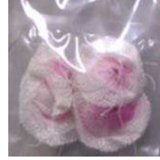
Figure 2. Lantern mantle (CAPTAIN STAG M-7911) used as our thorium source; overall, 50 pieces of mantle were used.
