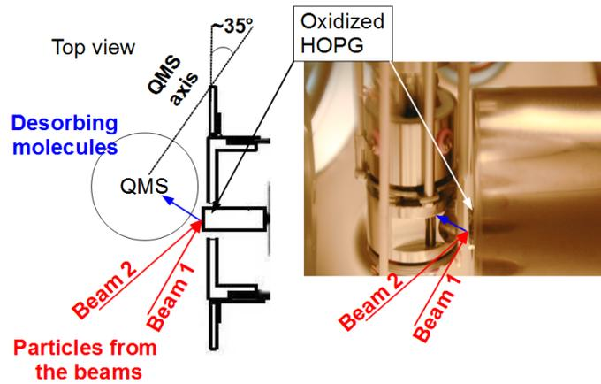
**Fig. 2.** Schematic top and side views (photo) showing the QMS and the cold surface configuration. The DED and TP-DED methods are indicated by red arrows (incoming particles from the beam lines) and by the blue arrow, which represents the fraction of desorbing species that are detected during the exposure phase. Adapted from Minissale (2014).
