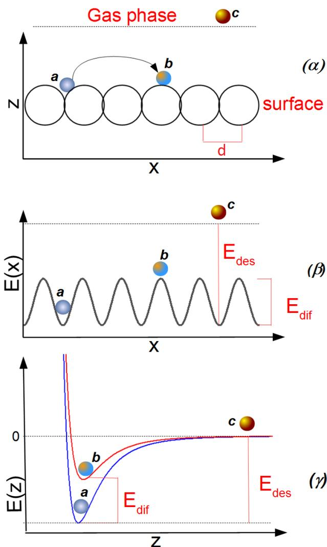
**Fig. 1.** (α): Schematic diagram of a substrate (black circles) with lattice constant  $d$ . (β): potential energy of adparticles on a surface in the  $x$  direction. (γ): potential energy of adparticles on a surface along the  $z$  direction. Particle (a) represents an adparticle in an adsorption site, particle (b) is in a transition state between two adsorption sites, and particle (c) represents a species in gas phase.
