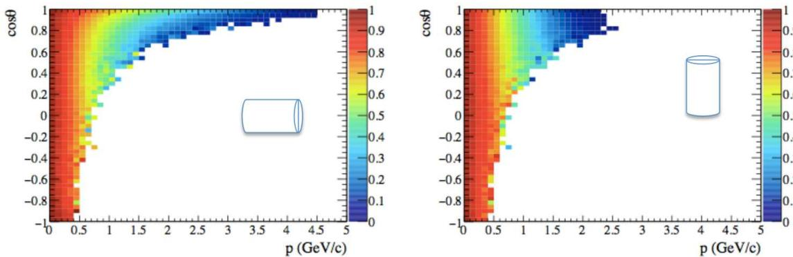
**Fig. 3.** The muon reconstruction efficiency as a function of muon momentum and angle to the neutrino beam axis for the two proposed detector orientations. The muon is required to stop within the detector for it to be reconstructed.
