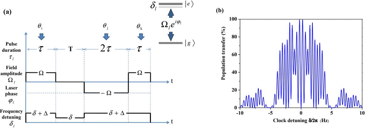
**Figure 3.** (color online). (a) Sequence of composite pulses  $\theta_i - T - \theta_j, \theta_k$  with specified laser parameters including detuning  $\delta_l$ , complex field amplitude  $\Omega_l e^{i\varphi_l}$ , pulse duration  $\tau_l$  where  $l = i, j, k$  and a free evolution time  $T$  between pulses. (b) Generalized Hyper-Ramsey resonance generated by composite pulses.
