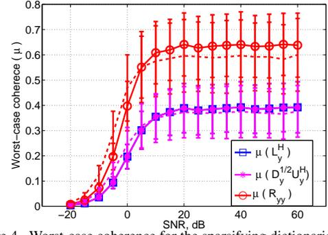
Figure 4. Worst-case coherence for the sparsifying dictionaries  $L_y^H$ ,  $D_y^{\frac{1}{2}} U_y^H$  and  $R_{yy}$  versus input SNR for UPDP with  $v = 8$  and  $N_f = 80$ . Dashed lines represent the coherence of the corresponding circulant approximation for  $D_y^{\frac{1}{2}} U_y^H$  (i.e.,  $Q^H$ ) and  $R_{yy}$  (i.e.,  $\bar{R}_{yy} = QQ^H$ ).
