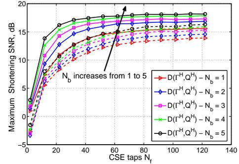
Figure 5. Maximum shortening SNR versus CSE taps for UPDP CIR with  $v = 5$ , SNR = 20 dB. Solid lines represent the  $D(I^H, Q^H)$  approach while the dashed lines represent the “significant-taps” approach proposed in [12].
