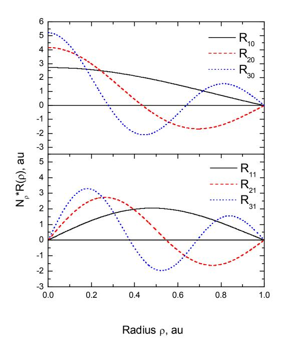
Fig. 1. The normalized functions  $R_{lm}(\rho)$  for some quantum numbers *l* and *m*. The radius of the cylindrical potential well is  $R_0=1$  au.
