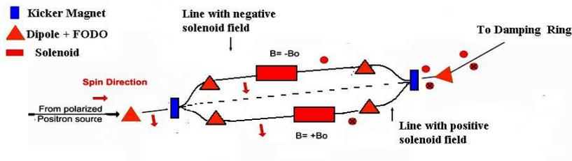
Figure 2: The schematic layout of the positron transport to Damping Ring with a two parallel lines spin rotator section.
