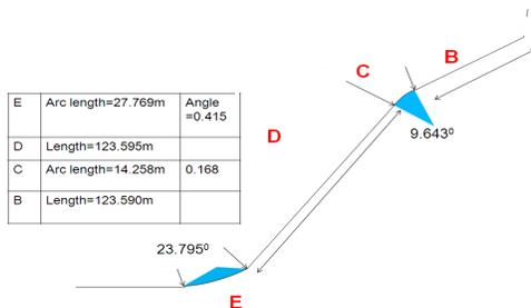
Figure 1: Schematic layout of new PLTR section
