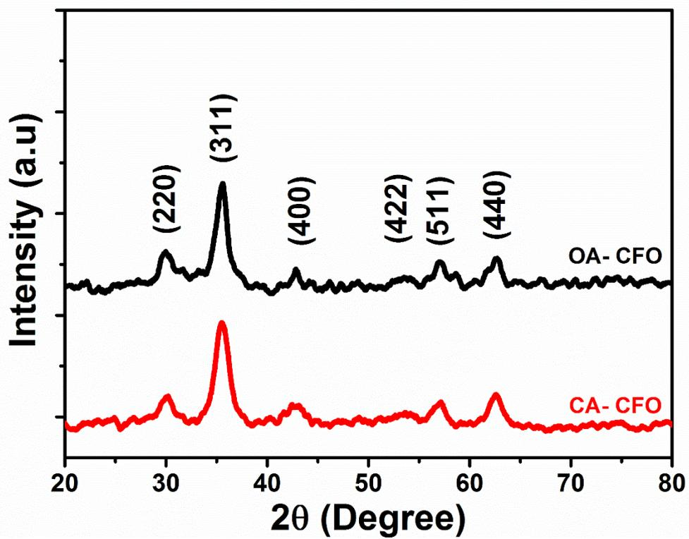
Fig. 1 X-ray diffraction patterns of OA-CFO and CA-CFO nanoparticles.
