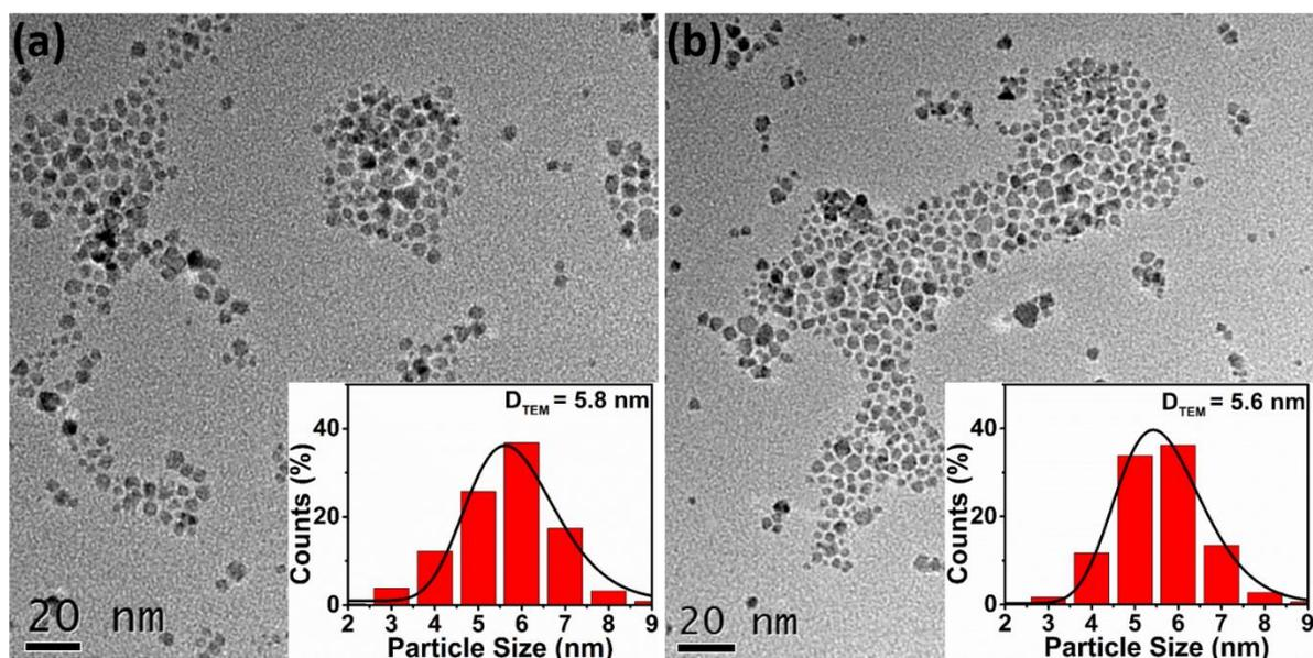
Fig. 2. TEM images of (a) OA-CFO nanoparticles and (b) CA-CFO nanoparticles. The inset in the figure shows distribution of particle size and its log normal distribution fit.
