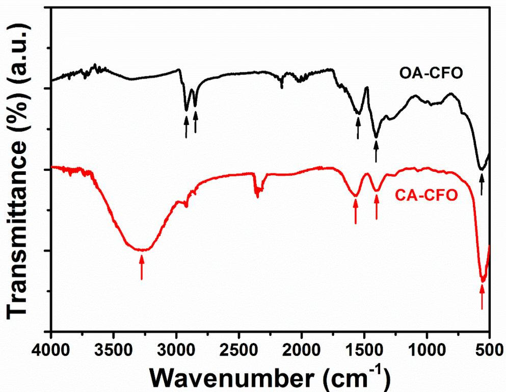
Fig. 4. FTIR spectra of OA-CFO and CA-CFO nanoparticles. Arrows marked OA-CFO spectra corresponds to  $2990 \text{ cm}^{-1}$ ,  $2850 \text{ cm}^{-1}$ ,  $1538 \text{ cm}^{-1}$ ,  $1410 \text{ cm}^{-1}$  and  $590 \text{ cm}^{-1}$  (from left to right) whereas the arrows marked to CA-CFO spectra corresponds to  $3275 \text{ cm}^{-1}$ ,  $1575 \text{ cm}^{-1}$ ,  $1405 \text{ cm}^{-1}$  and  $590 \text{ cm}^{-1}$  (from left to right).
