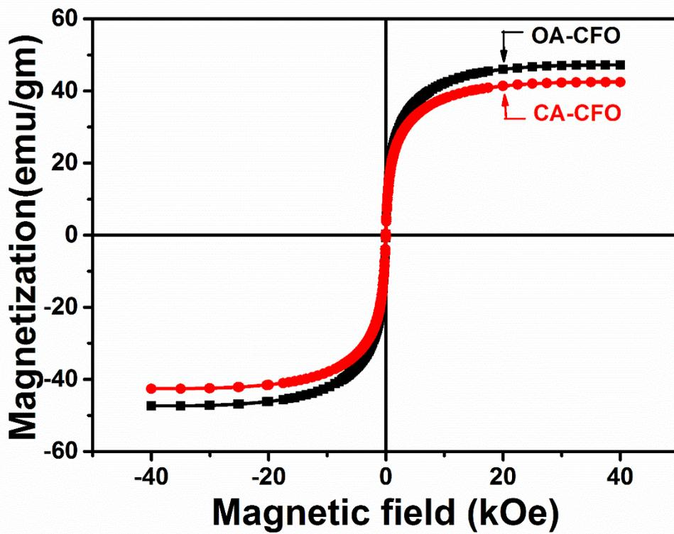
Fig. 3. Magnetic hysteresis loops for OA-CFO and CA-CFO nanoparticles at room temperature.
