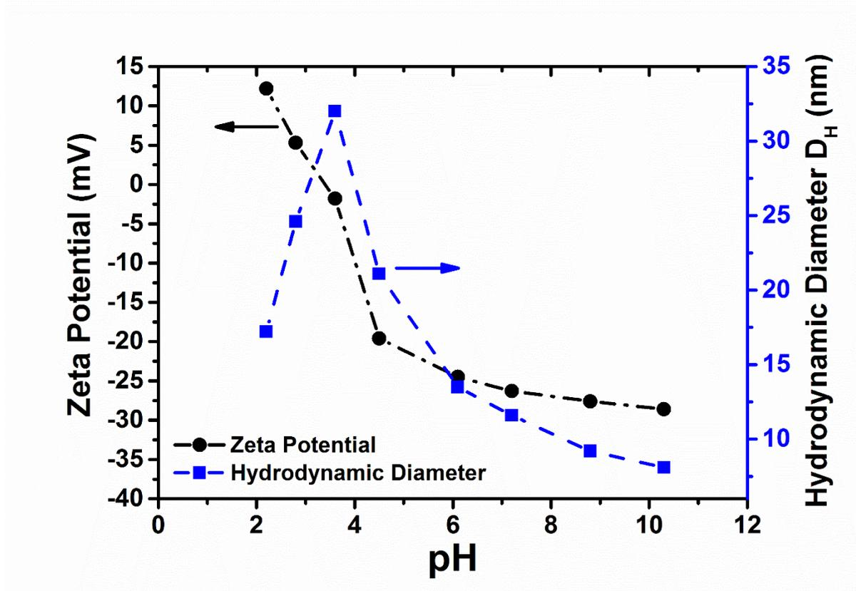
Fig. 5. Zeta potential and hydrodynamic diameter as a function of pH for CA-CFO nanoparticles.
