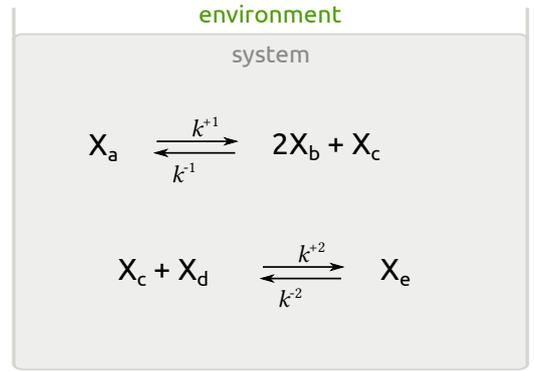
FIG. 1: Representation of a closed CRN. The chemical species are  $\{X_a, \dots, X_e\}$ . The two reaction pathways are labeled by 1 and 2. The nonzero stoichiometric coefficients are  $-\nabla_{+1}^a = -1$ ,  $\nabla_{-1}^b = 2$  and  $\nabla_{-1}^c = 1$  for the first forward reaction and  $-\nabla_{+2}^c = -1$ ,  $-\nabla_{+2}^d = -1$  and  $\nabla_{-2}^e = 1$  for the second one. Since the network is closed, no chemical species is exchanged with the environment.
