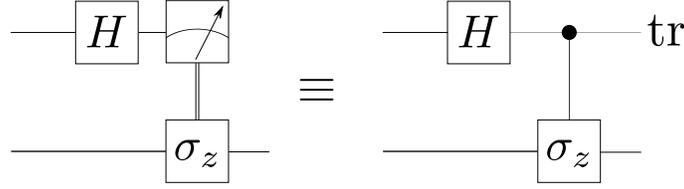
FIG. 7. Since we assume single qubit operations to be ideal, erasing a qubit through a rotation, measurement, and a conditional rotation is equivalent to rotating it, performing a CZ operation, and tracing over the qubit.
