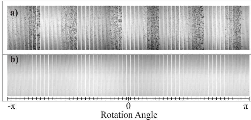
Fig. 3. Examples of the surfaces that result from (a) brittle and (b) ductile modes of material removal while diamond turning  $\text{LiNbO}_3$ . Each images are the composition of 59 images each taken at one specific angle.
