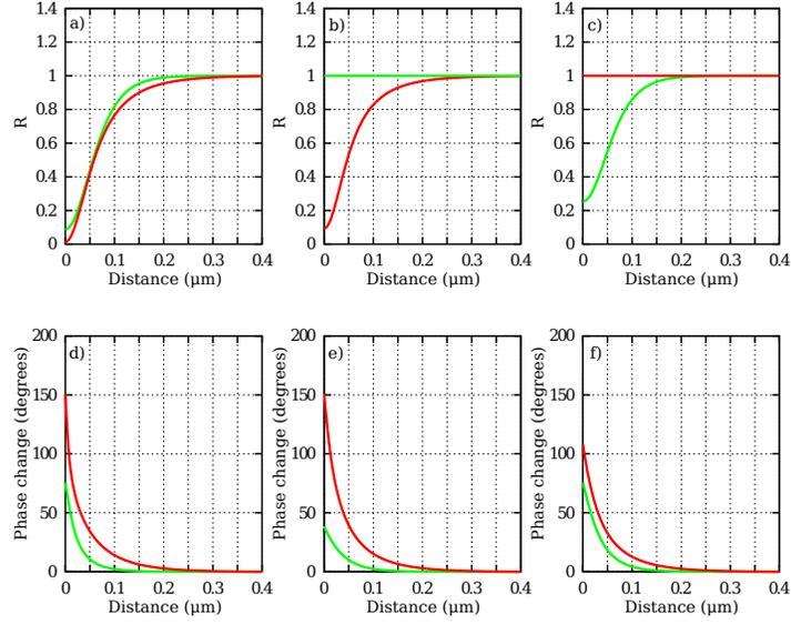
Fig. 10. Reflectivity  $R$  versus distance  $L$  between the prism and the resonator for 1064 nm (red) and 532 nm (green) for the SF11 prism (a), the red calcite (b) and the green calcite prism (c), and phase shift versus distance due to the reflection for the SF11 prism (d), the red calcite (e) and the green calcite prism (f).
