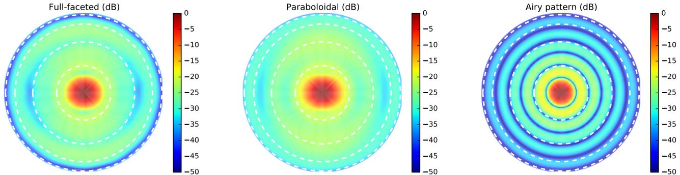
FIG. 3.— Simulated dish power patterns (NS polarization) at 137 MHz (see Sec. 2.2) with  $h_{\text{feed}} = 5$  m using the full-faceted model (left) and the perfect paraboloidal model (middle) are shown beside an ideal Airy pattern for a 14 m diameter dish for comparison. Dashed lines mark zenith angles of  $20^\circ$ ,  $40^\circ$ ,  $60^\circ$ , and  $80^\circ$ .
