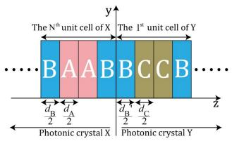
Fig. 1. Proposed 1-D photonic crystal model constructed by connecting two 1-D photonic crystals X and Y (X+Y), where X and Y contain *N* unit cells. For both X and Y, their thickness is given by Eq. 1, and a single layer of A (or C) is sandwiched between half layer of B. Additionally, A and C has a small differences of refractive index.
