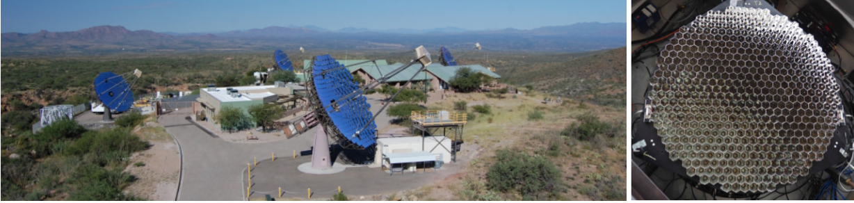
Fig. 1.— The VERITAS array in Arizona (left) and the PMT camera of a single telescope (right), that covers a total field-of-view of diameter 3.5^\circ . The hexagonal reflective light cones reduce the dead space between the circular PMTs.
