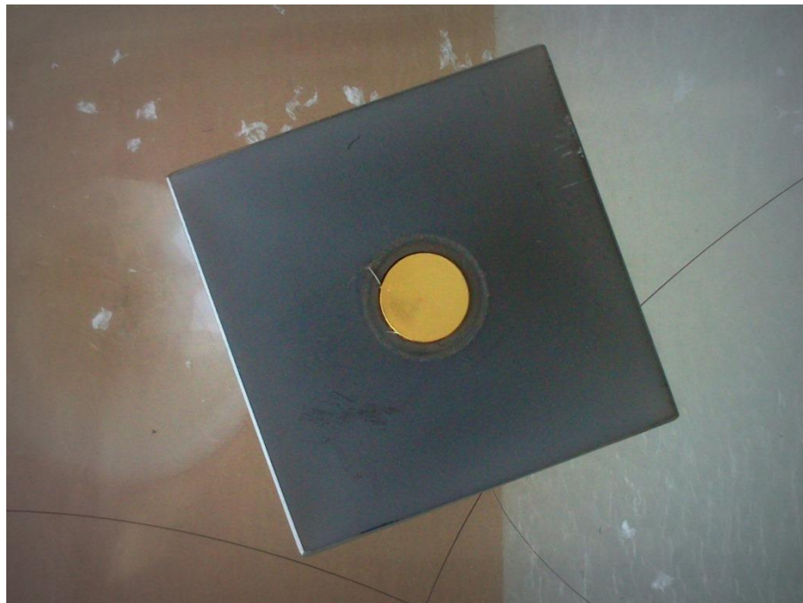
Figure 33: View of a TM mock-up (0.0096 kg). The central part is the Au/Pt gold coated insert.
