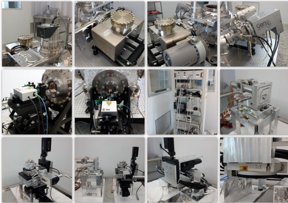
Figure 31: From the top left: turbo-molecular pump, ionic pump, ionic and scroll pumps, plasma, 2 views of the interferometer, electronics rack, support system (needles), RTmu and the actuators that allow to change its position/attitude, support system together with the RTmu, actuators of the pivot of the pendulum with a detailed view.
