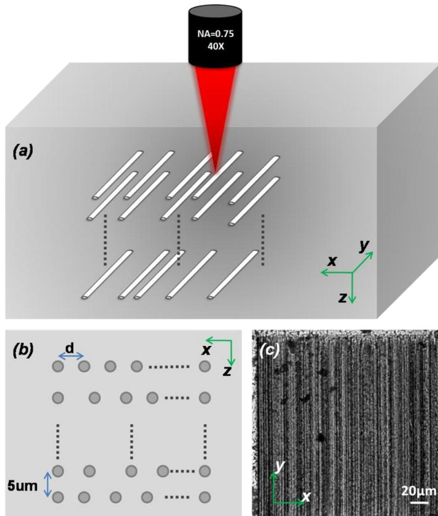
**Figure 1:** Fabrication details. The scattering rod photonic lattice is fabricated in the bulk of the glass by direct laser writing as illustrated in panel (a). The distribution of the lattice structure on the x-z plane is depicted in panel (b). An optical transmission micrograph of a fabricated rod lattice is shown in panel (c).
