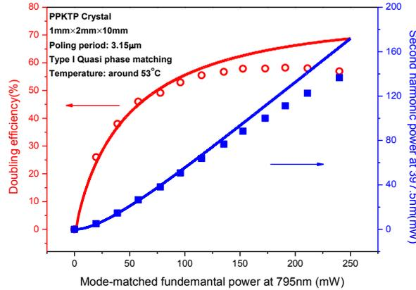
**Figure 2** Frequency doubling results for the 20 mm-long PPKTP crystal. Blue squares are the measured SH power at 397.5 nm, red circles are the corresponding doubling efficiency, and lines are the calculated result.
