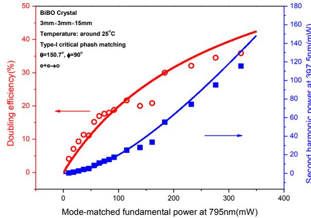
**Figure 4** Frequency doubling results for the 15 mm-long BiBO crystal. Blue squares are the measured SH power at 397.5 nm, red circles are the corresponding doubling efficiency, and lines are the calculated results.
