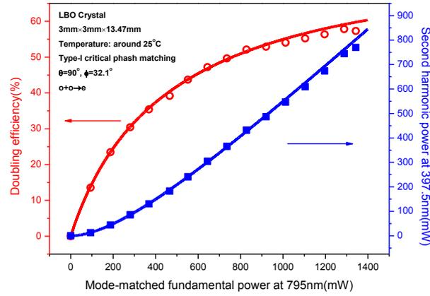
**Figure 3** Frequency doubling results for the 13.47 mm-long LBO crystal. Blue squares are the measured SH power at 397.5 nm, red circles are the corresponding doubling efficiency, and lines are the calculated result.
