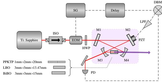
**Figure 1** The schematic diagram of the frequency doubling system. ISO: optical isolator; EOM: phase-type electro-optical modulator; HWP: half-wave plate; PZT: piezoelectric transducer; PD: photodiode; SG: signal generator; DBM: double balanced mixer; LPF: low-pass filter. Solid lines are the optical parts, and the dash lines are the electric parts used to lock the cavity.
