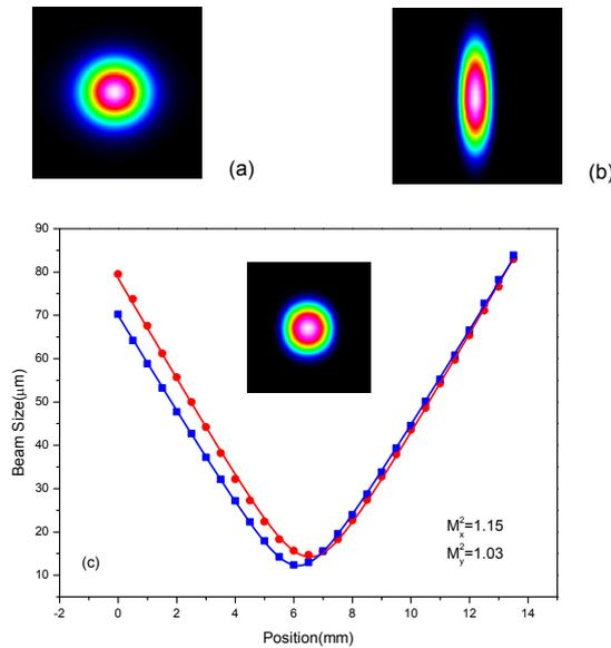
**Figure 6** Typical intensity distribution of the output UV beam and the measured  $M^2$  of the LBO cavity. (a). Typical intensity distribution of the PPKTP cavity output beam; (b). Typical intensity distribution of the LBO cavity output beam, elliptical in shape; (c). Measured  $M^2$  of the LBO cavity output after shaping, the inset is the intensity distribution after the anamorphic prism pair.
