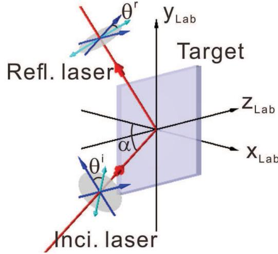
Fig. 1. A plane wave laser pulse obliquely incident onto a plane plasma target in the lab system. Blue axes, the  $p$ - and the  $s$ -polarization axes. Cyan two-ended arrows, polarization direction or major axis of polarization ellipse. See text for symbol meanings.
