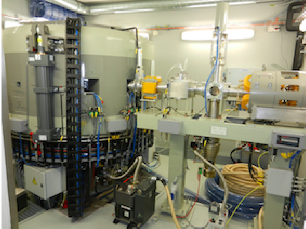
Figure 1.5: The 18 MeV proton cyclotron installed at the Inselspital in Bern in the framework of the SWAN project. One of the out-ports for radioisotope production are visible together with the characteristic beam transfer line for research activities.
