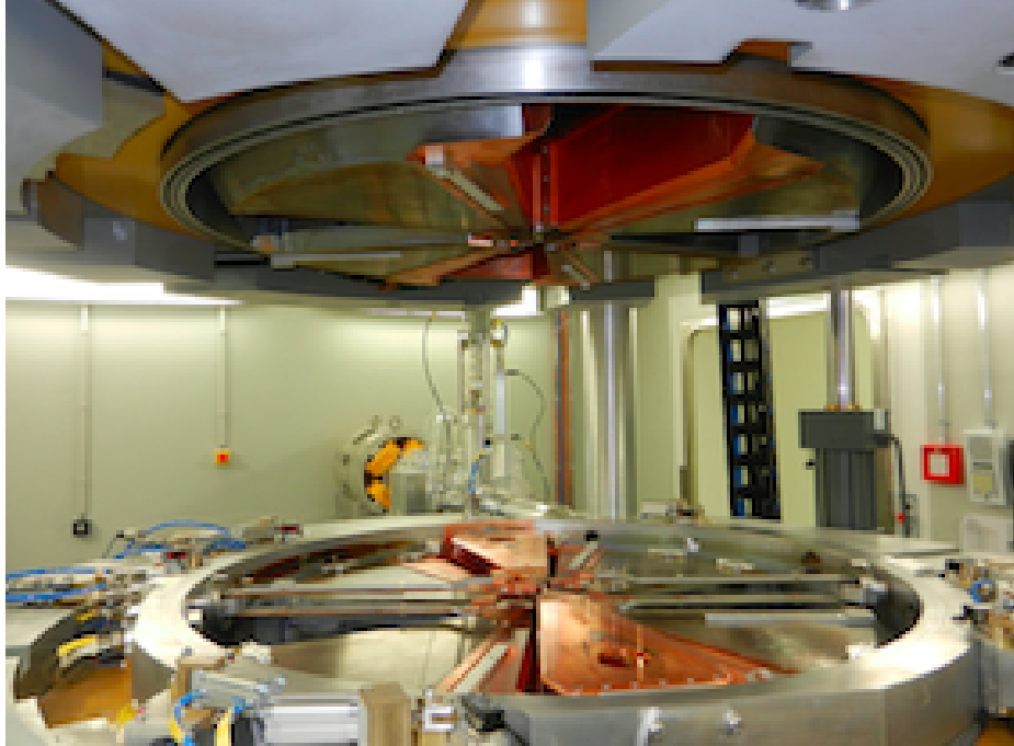
Figure 2.10: The Bern cyclotron opened during commissioning. The 30^\circ dees are visible together with the magnetic poles producing the alternating magnetic field for vertical focussing ( hills and valleys ). The two flaps for the D^- operation mode and some of the eight exit ports are also visible together with the targets for ^{18}\text{F} production. The exit port number four is connected to the BTL whose first quadrupole doublet is located in the cyclotron bunker.
