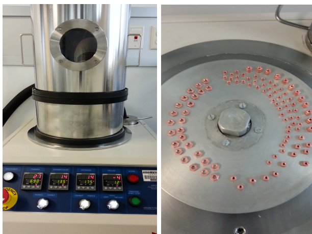
Figure 3: Parylene coating of copper nuts. Left: the parylene coater. Right: parts on the deposition stand.
