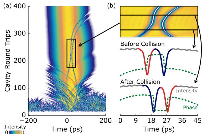
FIG. 7. Radiation build-up dynamics (using the parameters as in Fig. 2, but initiated from a different randomized shot noise field): (a) temporal evolution; (b) magnified collision region and dark soliton profiles within the bright pulse, before and after a collision at 200 and 240 round trips, respectively (color is used to identify each soliton).
