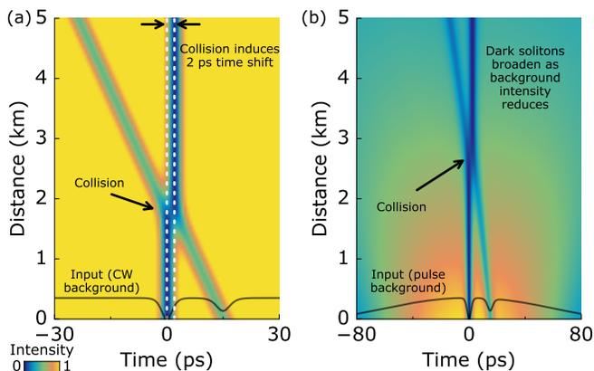
FIG. 6. Collision dynamics between a black  $|B| = 1$  and gray  $|B| = 0.6$  soliton in transmission: (a) on a CW background (white dotted lines indicate the collision-induced temporal displacement of the black soliton); (b) on a bright pulse background.
