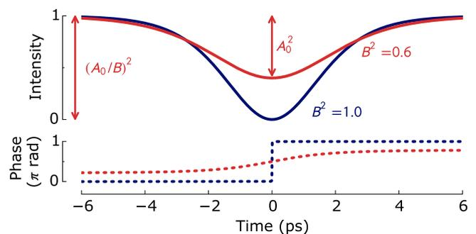
FIG. 3. Definition of dark soliton, showing the intensity and phase of a black ( $|B| = 1$ ) and a gray ( $|B| = 0.6$ ) soliton. The notation of Eqn. 2 is illustrated by arrows, which relate to the gray soliton.
