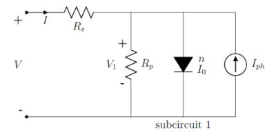
Figure 1: One diode model of a solar cell.
