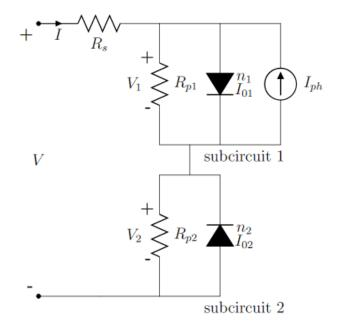
Figure 6: Two diode model of a solar cell, as in references [11, 12]. Subcircuit 1 has the photocurrent source, and a diode with reverse saturation current  $I_{01}$  and ideality factor  $n_1$ . Subcircuit 2 has a reverse bias diode and a shunt resistance.
