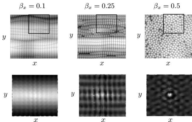
FIG. 5: Top-view surface morphologies (top row) predicted by Eq. (10) at  $t = 1000$  for  $\alpha_x = 0.5$ ,  $r_0 = 5$ , and different values of  $\beta_x$  (see legends). Corresponding normalized autocorrelation functions (bottom row) computed over the indicated squares of size  $100 \times 100$ .
