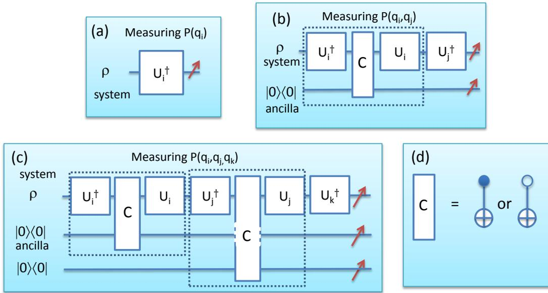
**Figure 4.2:** Circuits for measuring SEP (a), and two-time JP (b), and three-time JP (c). The grouped gates represent measurement in  $\{\Pi'_0, \Pi'_1\}$  basis. The operation  $C$  can be either CNOT gate or anti-CNOT gate, as described in the text. In (c) the second CNOT gate is applied between first and third spin. The pointer at the end in each circuit represents the measurement of diagonal elements of the density matrix. (d) Block  $C$  represents either CNOT or anti-CNOT gate.
