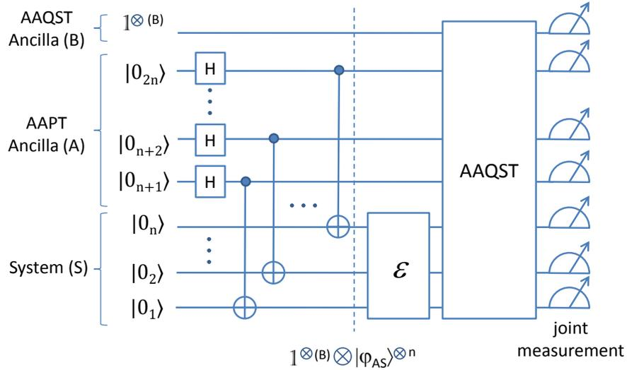
**Figure 3.2:** Quantum circuit for SSPT. Building blocks of the circuit involves initialization of the system and ancilla registers, encoding of the input states into subspaces of system-ancilla register, application of process  $\mathcal{E}$ , and finally AAQST.
