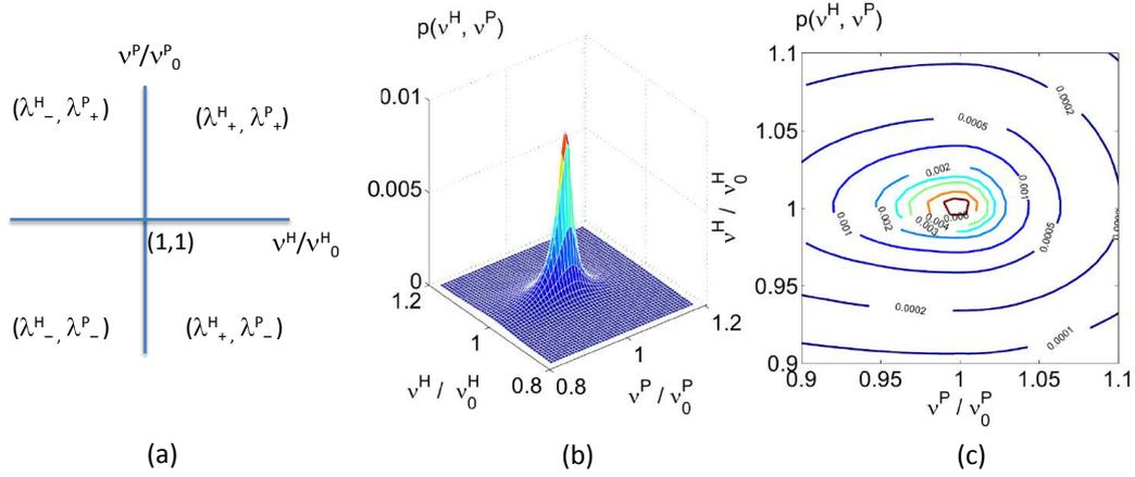
**Figure 5.6:** Characterization of RFI correlations between  $^1\text{H}$  and  $^{31}\text{P}$  channels of QXI probe. (a) The  $\nu^H - \nu^P$  plane, (b) the surface plot of the RFI profile  $p(\nu^H, \nu^P)$ , and (c) the contour plot of  $p(\nu^H, \nu^P)$
