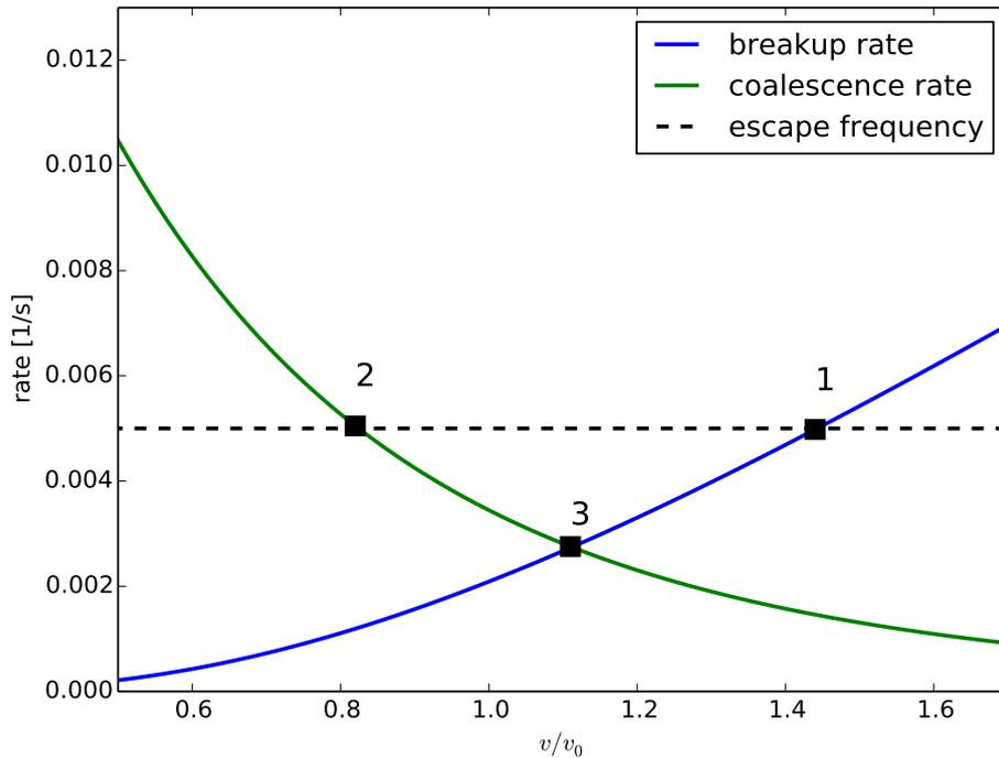
Figure 1: Stable solution to optimization of PBE source terms are located around points indicated with squares. . ‘1’ corresponds to pure breakup solution, ‘2’ is pure coalescence, ‘3’ is balanced solution.
