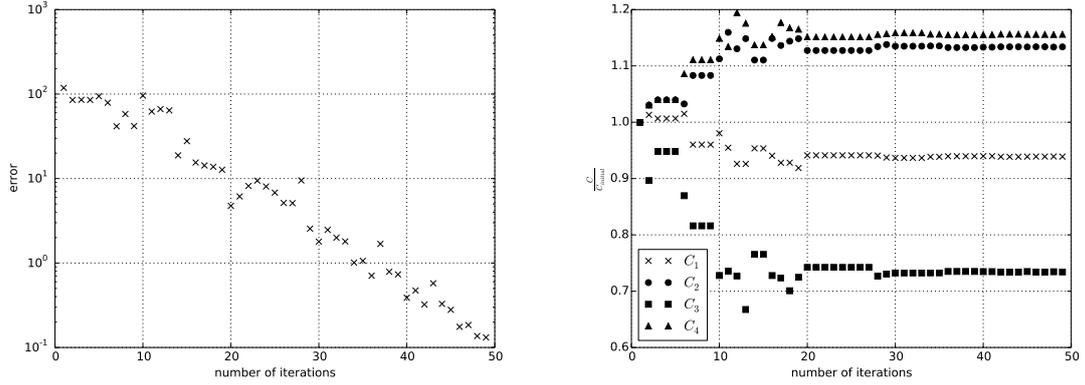
Figure 2: Rate of convergence of optimization process. Left-hand side plot shows error as defined by Eq. 15 as a function of number of iterations. The second plot shows relative change in  $C_1$ – $C_4$  parameters being optimized.
