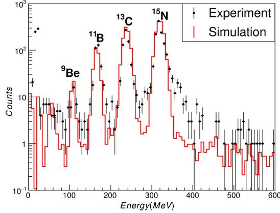
Figure 6: The spectra of energy deposition in a 7 mm thick detector layer. The black points are the beam test results and the red solid line is correspond simulation.
