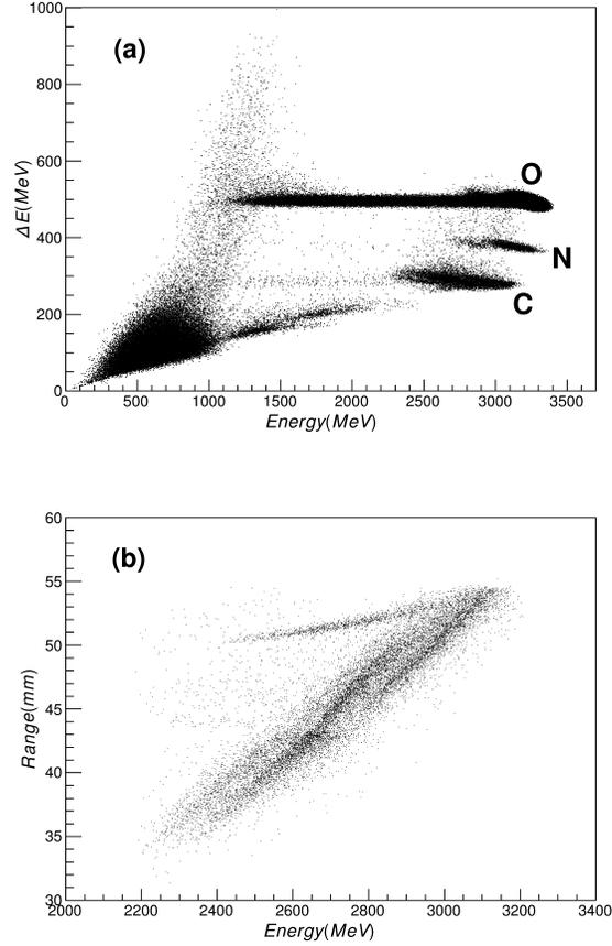
Figure 1: The PID spectra of the detector through Monte Carlo simulation with 2% energy resolution for each layer of the telescope. (a) is the PID spectrum through  $\Delta E - E$  method while (b) is the PID spectrum for Carbon isotopes through  $Range - E$  method.
