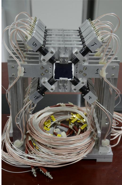
Figure 2: Prototype of the multi-layer CsI(Tl) telescope.
