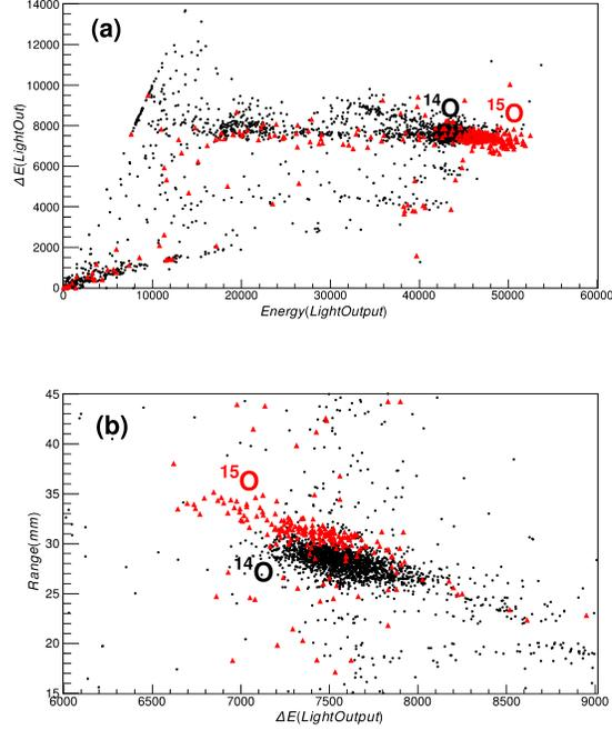
Figure 7: The PID spectrum for Oxygen Isotopes in the detector. (a) is the spectrum through  $\Delta E - E$  method while (b) is the spectrum through  $\text{Range} - \Delta E$  method.
