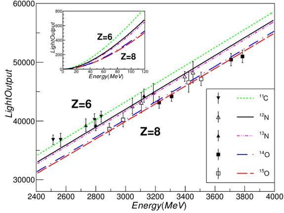
Figure 5: Total light output against the energy for different incident particles in all of the crystals. The symbols are experimental data. The different curves are the result of a least-squares fit to Eq.(9) in Ref [32]. The inset picture shows the curves in the low energy region.
