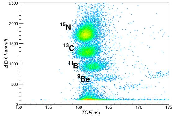
Figure 4: The spectrum of energy deposition against time of flight for the secondary beam.
