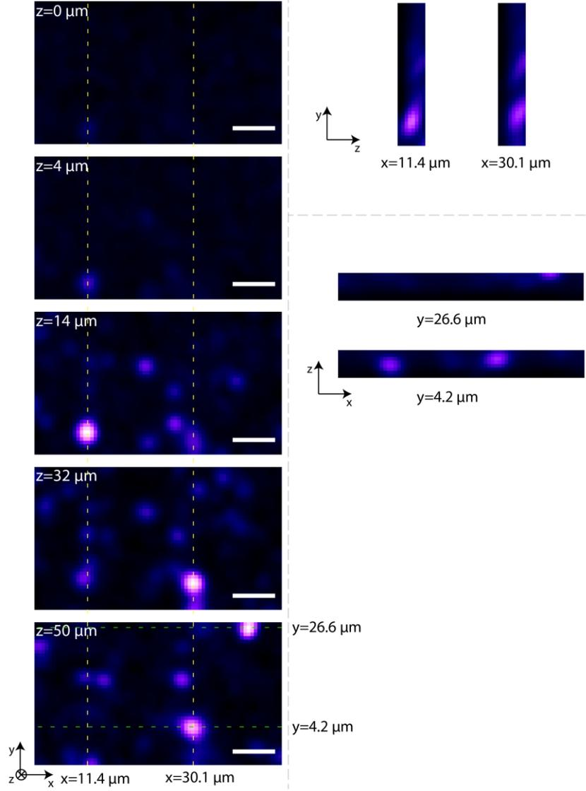
Fig. 4. Two-photon images of fluorescent beads.  $(y,x,z)$  Field of view is  $28 \times 49 \times 50 \mu\text{m}$ . Scale bars are  $10 \mu\text{m}$ . To view all the frames see Media 1.
