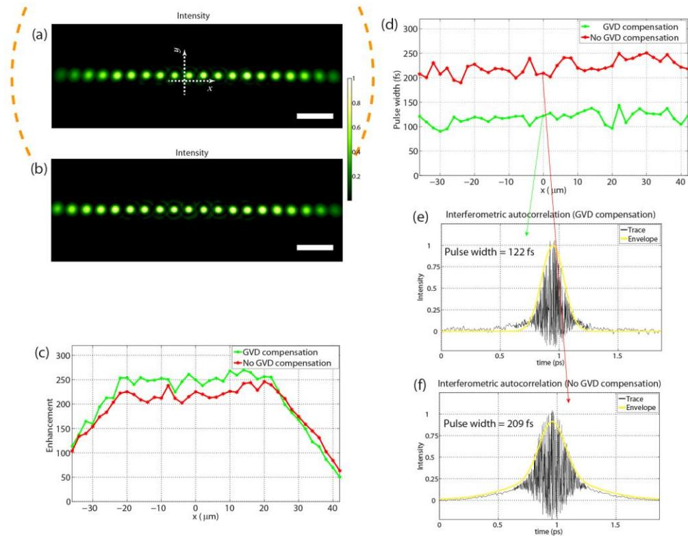
Fig. 3. Pulse width characterization. Intensity of the generated focused pulses at 800 nm without (a) and with (b) GVD compensation. (c) Intensity enhancement vs position. (d) Pulse width vs position. (e), (f) Sample interferometric autocorrelation traces of the central focused pulses with and without GVD compensation respectively. Scale bars are 10  $\mu\text{m}$ . The dashed orange semi-circle represents the core of the multimode fiber.
