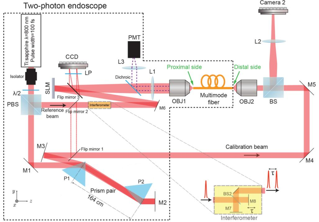
Fig. 8 Complete diagram of the experimental setup.
