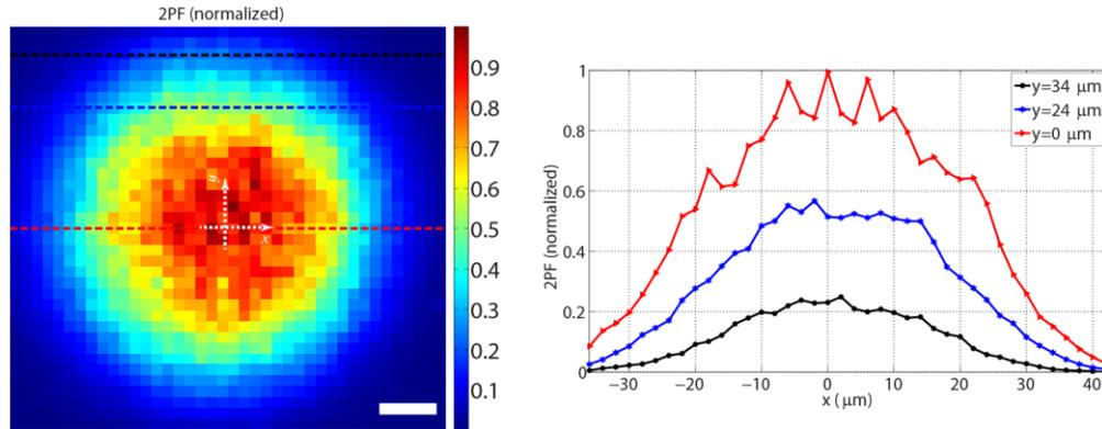
Fig 5. Normalized fluorescent photons as a function of position. Scale bar is 10  $\mu\text{m}$
