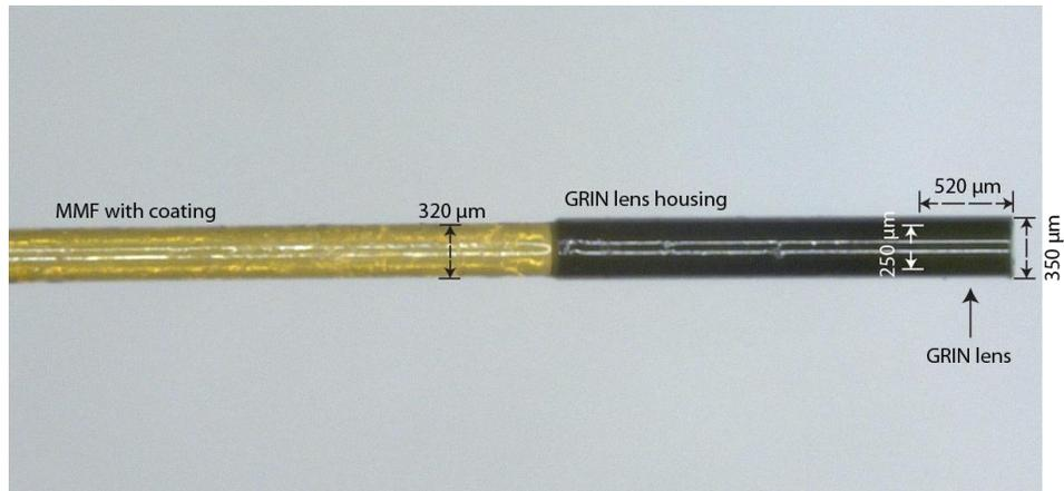
Fig. 7. Multimode fiber probe. The white horizontal lines are the reflection of the lamp of the microscope.
