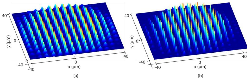
Fig. 6. Experimental PSF of the multimode fiber imaging system. (a) Single-photon fluorescence. (b) Two-photon fluorescence.
