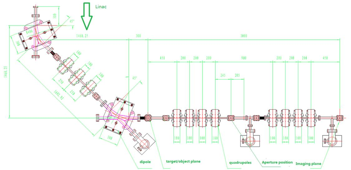
Fig.1. the layout of the eRad beam line based on THU linac
