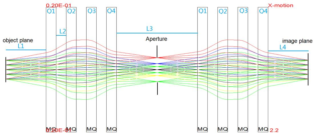
Fig.3. the beam trajectory of the triplet imaging system in X direction.
