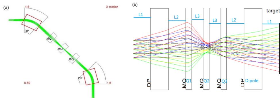
Fig.3. Achromat with beam angle and position calibration on the target in x direction according to doublet imaging system optical (a) and beam trajectory (b).
