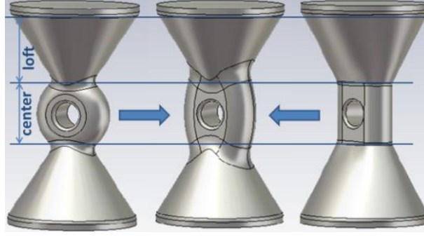
Fig. 2. Three types of inner conductors: ring shaped (left), elliptical shaped (medium) and race track (right).
