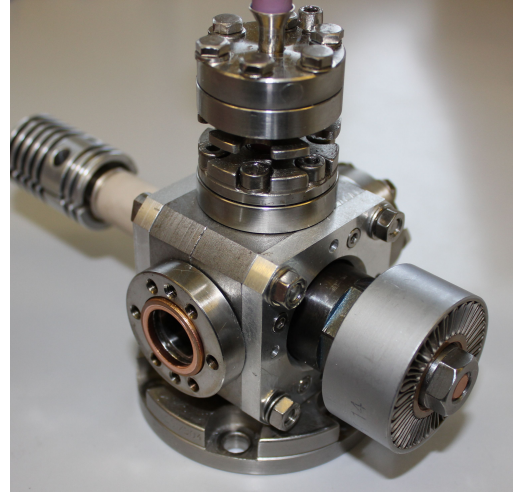
FIG. 4: (Color online) General view of the MaMFIS with the radial extraction of ions. Device with water cooling collector for dissipation power of up to 1 kW (left photo) and with air cooling collector for dissipation power of up to 300 W (right photo).
