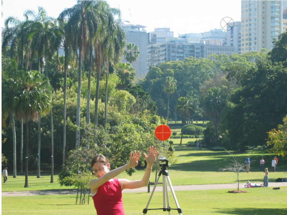
Figure 2. A QUT student performing the parallax experiment. The display of nine fingers indicates that the photo is the 9 th image in the sequence. In this case the target was 7.8 m away from the camera baseline. The diagonal cross in the circle in the top right of the picture is the origin used for calculating the parallax.
