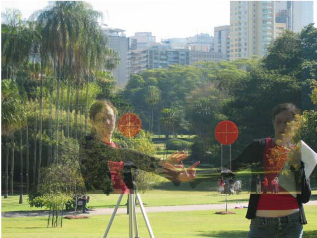
Figure 4. Two photos have been overlaid by matching the distant background to enable direct measurement of the horizontal distance between the target in the two images.
