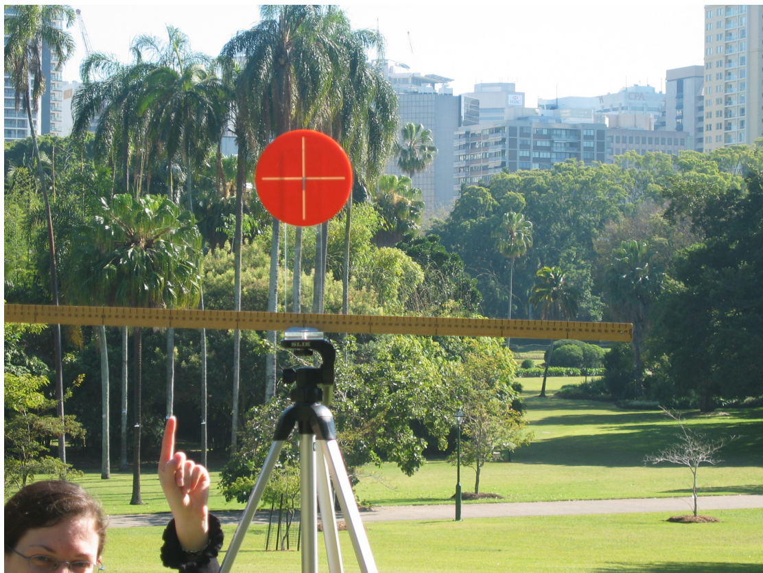
Figure 2. Photo of a metre rule on a tripod for obtaining the physical size of the CCD pixels in the camera.
