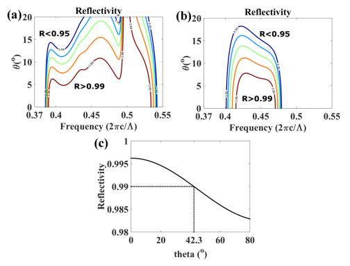
Fig. 3. (a) Reflectivity contour as a function of frequency and incident angle with the parameters  $h_1 = 0.685\Lambda$  and  $h_2 = 0.45\Lambda$ . (b) Reflectivity contour as a function of frequency and incident angle with the parameters  $h_1 = 0.685\Lambda$  and  $h_2 = 0$  (HCGs). (c) Reflectivity as a function of incident angle at a frequency of  $0.5 \times 2\pi c / \Lambda$ . The high reflection angle region is significantly expanded because of the slab waveguide modes.
