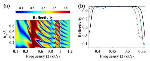
Fig. 2. (a) Reflectivity contour as a function of frequency and grating-layer thickness with  $h_1 = 0.685\Lambda$ . The thick grating layer can sustain WGA modes, which are essential for HCGs. The interference among guided modes, WGA modes, and Fabry-Perot modes leads to the broadband high reflection (dark red area). (b) Reflectivity with the parameters described in (a) for three different configurations:  $h_2 = 0.45\Lambda$  and  $\eta = 0.5$  (black line),  $h_2 = 0.5\Lambda$  and
