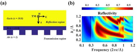
Fig. 4. (a) Schematic of the asymmetric waveguide structure. (b) Reflectivity contour of the structure with a substrate ( $\varepsilon_r = 10.9$ ) as a function of frequency and grating thickness with  $h_2 = 0.45\Lambda$ .
