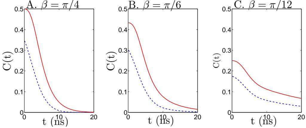
Fig. 8: Evolution of the coherence ratio  $C(t) = \frac{|\rho_{e_1, e_2}|}{\rho_{e_1, e_1} + \rho_{e_2, e_2}}$  of a critically damped V-system ( $\zeta \ll 1$ ). Here  $\bar{\gamma} = 1.0$  and  $\Delta = 1.0$ , but with varying pumping rate asymmetry  $\gamma_1 = \bar{\gamma} \sin^2(\beta)$  and  $\gamma_2 = \bar{\gamma} \cos^2(\beta)$  and dipole alignment,  $p = 1.0$  (solid) and  $p = 0.7$  (dashed).
