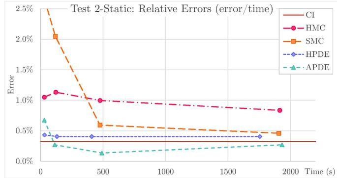
Table 7: Test 2-Static. In the first Table, the fair fee for the Heston model, with no ratchet or annual ratchet. In the second Table the run times for the no-ratchet case ( $\rho = -0.5$ ). Finally, the plot of relative error (w.r.t. MC value) for the three methods in the case  $\rho = -0.5$  with no ratchet. The parameters used for this test are available in Table 2 and in Table 6.
