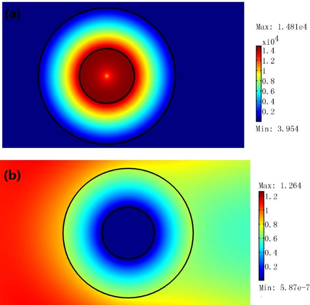
Figure 5| The 2D FEM simulation results for a TE wave case. We plot the absolute value of the electric field's  $z$  component. The open concentric ring resonator here has a subwavelength size (e.g.  $a=\lambda_0/15$ ,  $b=\lambda_0/6$ ). (a) A line current with amplitude 1A is set at the center of the concentric ring resonator. (b) A plane wave with unit amplitude is incident onto the resonator from the left.
