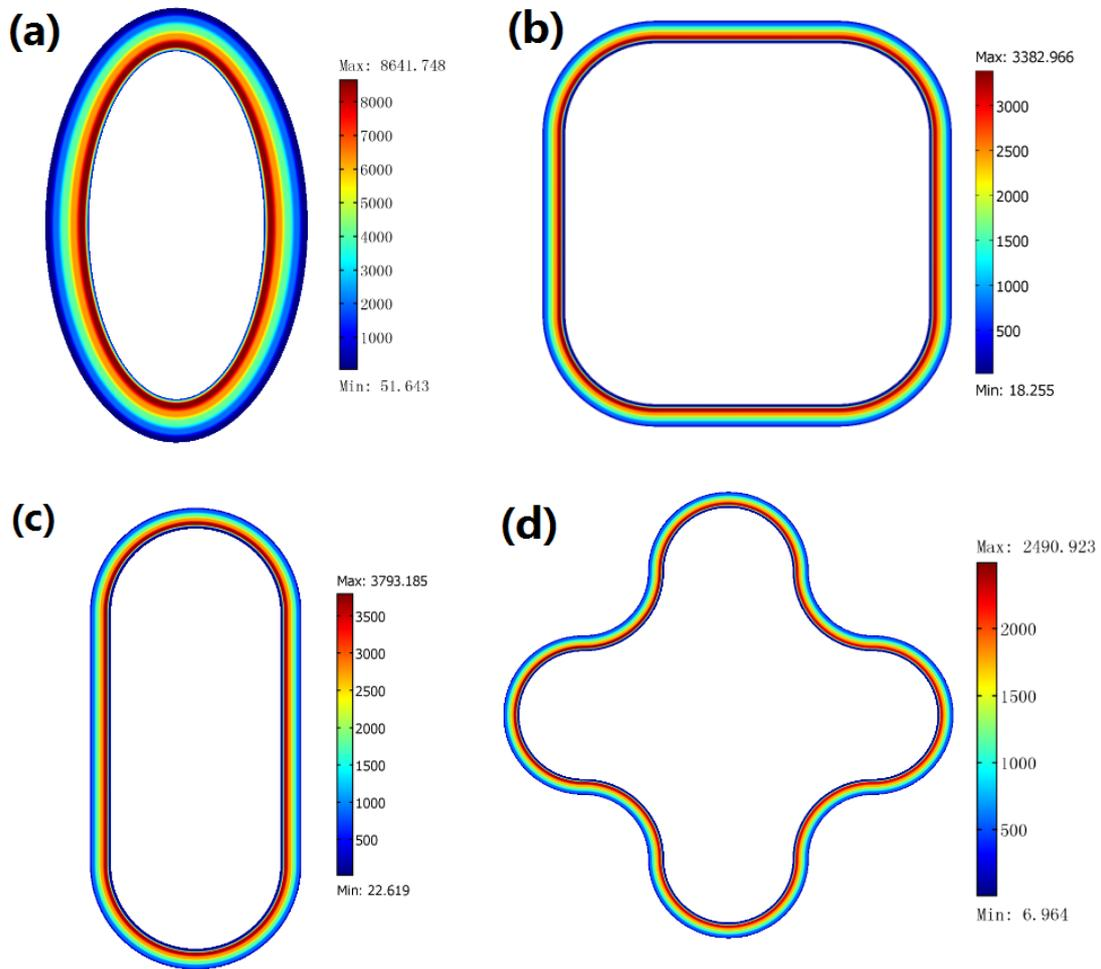
Figure 3| Some cavities of other shapes designed by the OST. We only plot the absolute value of electric field's  $z$  component inside the resonator for the TE polarization. We use one line current source with amplitude 1A inside the loop to excite the mode. (a) an elliptic resonator. (b) a rectangular resonator with smooth corners. (c) a playground shaped resonator. (d) a petaloid resonator. The whole size of these resonators are all smaller than the wavelength in above simulations.
