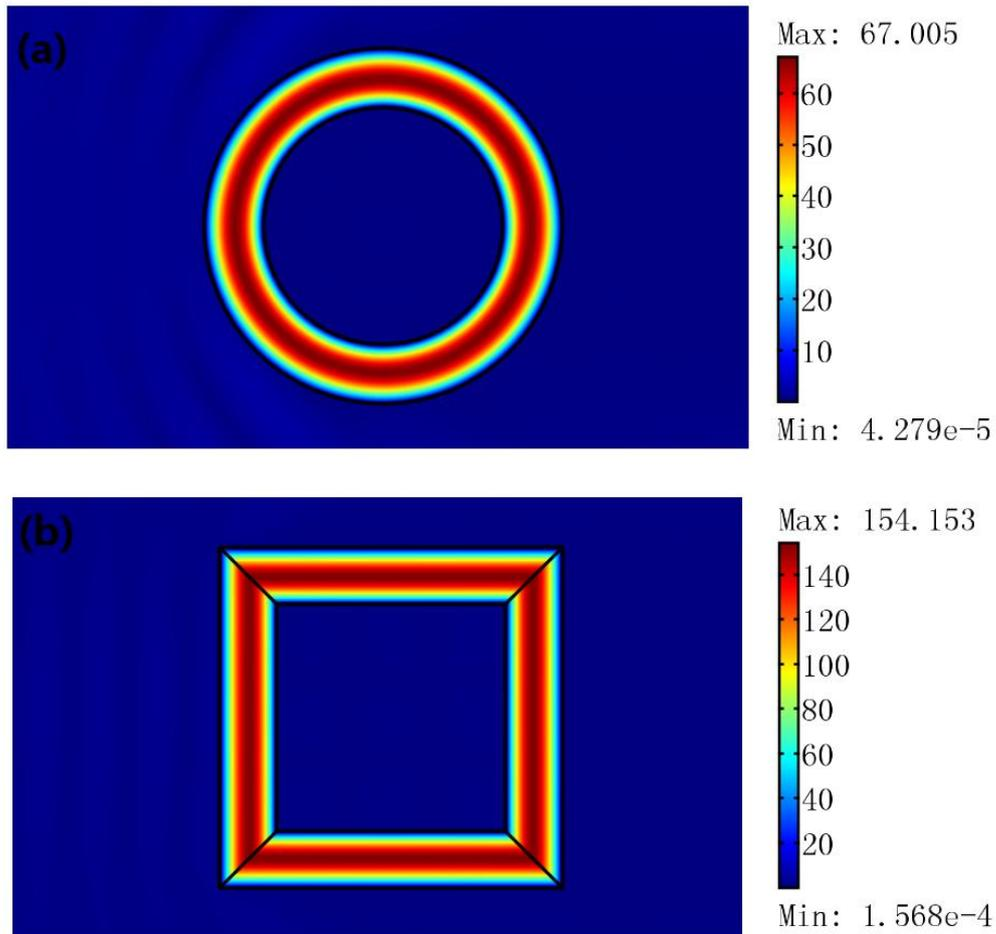
Figure 4| The 2D FEM simulation results for a TE wave case. A plane wave with unit amplitude is incident onto the resonator from the left. We plot the absolute value of the electric field's  $z$  component. (a) A concentric ring resonator with inner radius  $\lambda_0$  and outer radius  $1.5\lambda_0$ . (b) A rectangular ring resonator with inner side length of  $2\lambda_0$  and outer side length of  $3\lambda_0$ .
