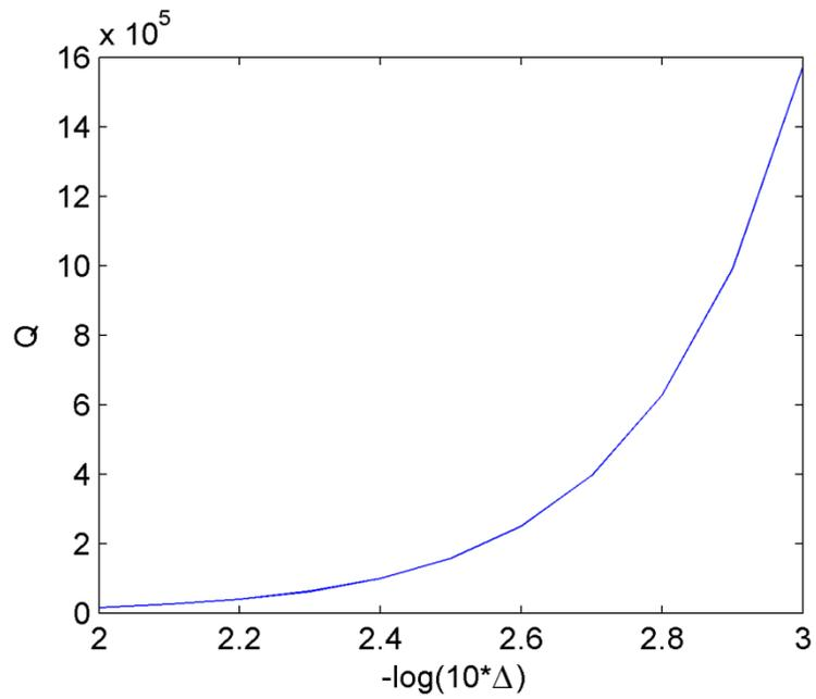
Figure 8| The FDTD simulation results: the relation between  $\Delta$  and the Q factor of the resonator. Here we set  $\mu_\theta=1/\Delta$ , and  $\mu_r = \epsilon_z = \Delta$  in a concentric ring resonator with size  $a=\lambda_0$  and  $b=1.5\lambda_0$ .  $\lambda_0$  is the resonance wavelength. If  $\Delta \rightarrow 0$  (e.g.  $-\log(10 \cdot \Delta)$  approaches infinity), the Q factor approaches infinity.
