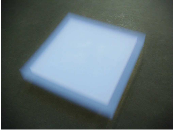
Fig. 1 Box-framing aerogel with a dimension of approximately 93 \text{ mm} \times 93 \text{ mm} \times 17 \text{ mm} (sample that is not contamination controlled; ID = TNPP s1-2b). The 0.03 \text{ g/cm}^3 layer, except the top surface, surrounds the 0.01 \text{ g/cm}^3 layer.
