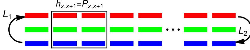
**Figure 8.** Schematic illustration of the degenerate boundary driven 3-color quantum chain, or spin-1 Lai-Sutherland chain. The incoherent boundary jump processes transform just a pair of colour states (red and blue), while the green states remain invariant and hence the number of green particles is a constant of motion.
