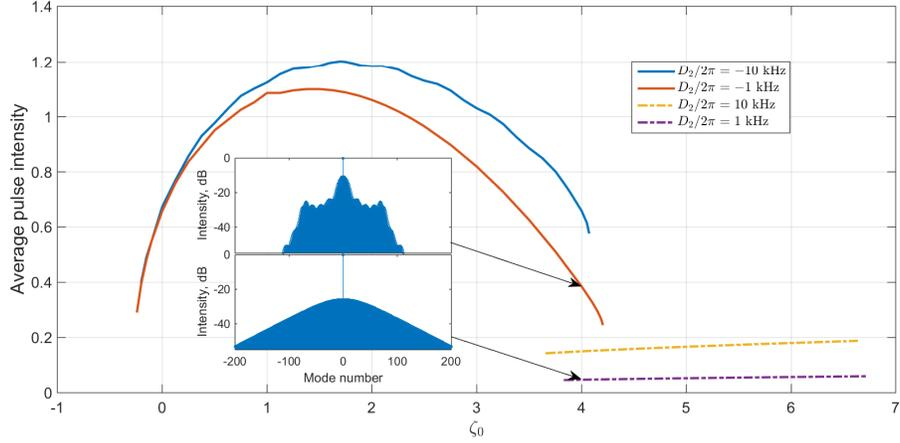
Fig. 6. Comparison of average pulse intensity for the same absolute values of normal ( $2\Delta/\kappa = 2$ ,  $P_{\text{in}} = 12.5\text{mW}$ ) and anomalous GVD combs. Insets show corresponding comb spectra.
