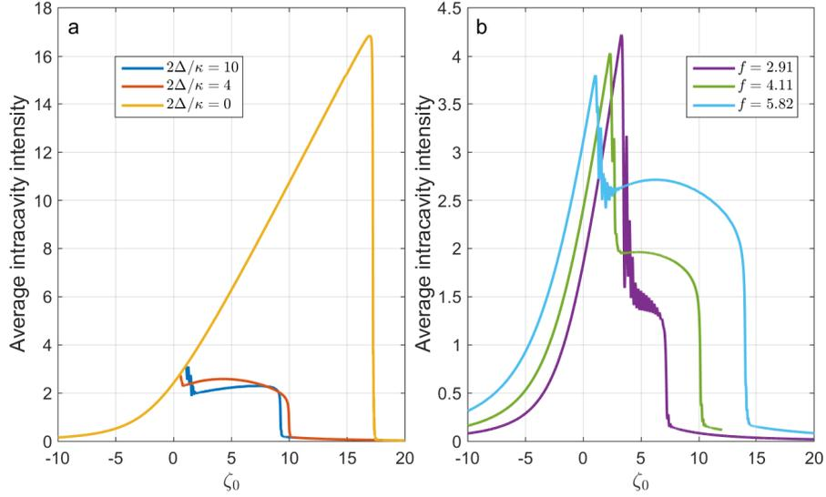
Fig. 1. Intracavity average intensity  $U$  vs. detuning  $\zeta_0$  in normal GVD microresonators. Left: Same input power, different perturbations for  $2\Delta/\kappa = 0$  (no comb) and  $2\Delta/\kappa = 4, 10$ .  $P_{\text{in}} = 50\text{mW}$ . Right:  $2\Delta/\kappa = 8$ ,  $P_{\text{in}} = 25, 50$  and  $100$  mW.
