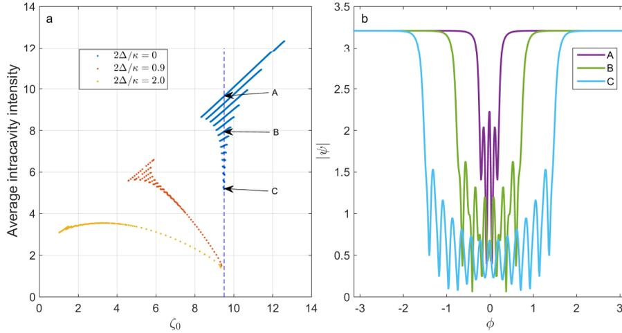
Fig. 4. Transition of discrete spectrum of dark solitons into continuous platicons upon increased perturbation  $\Delta$  of the pumped mode frequency at  $P_{in} = 50$  mW (left). Several higher order dark dissipative solitons (right).
