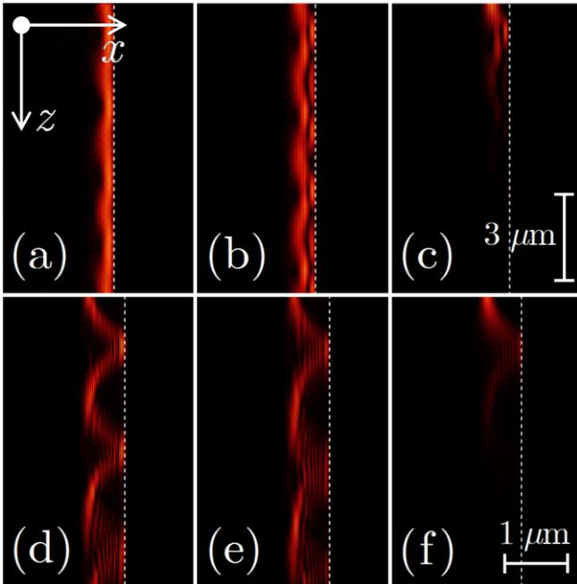
Fig. 6. Evolution of a beam launched into the second (a) and fifth (b),(c) waveguides in a truncated chirped subwavelength array with  $\delta d = 1.2 \text{ nm}$ . Evolution of a beam launched into the 25<sup>th</sup> waveguide for  $\delta d = 0.4 \text{ nm}$  (d) and  $0.8 \text{ nm}$  (e),(f). In (c),(f) metallic losses are taken into account. The propagation distance is  $10 \mu\text{m}$  and the width of the transverse window is  $3 \mu\text{m}$ . Dashed lines: position of the interface.
