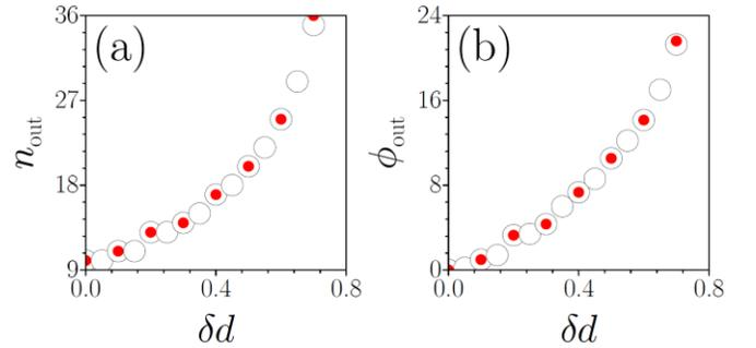
Fig. 3. Output waveguide number (a) and output propagation angle in degrees (b) versus chirp rate  $\delta d$  (in nanometers). Empty circles show dependencies obtained in the absence of metallic losses, while red dots correspond to the case with metallic losses. Total propagation distance is  $3 \mu\text{m}$ .
