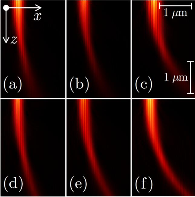
Fig. 4. (a)-(c) Same as in Figs. 2(d)-2(f), but for nonzero losses  $\alpha_m = -0.19$  in the metal region. In (d)-(f) gain  $\alpha_d = 0.04$  is added into dielectric layers. The propagation distance is  $3 \mu\text{m}$ , while the width of the transverse window is  $2 \mu\text{m}$ .
