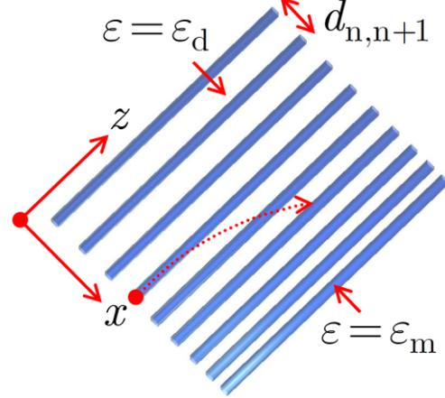
Fig. 1. Schematic representation of a chirped subwavelength array consisting of dielectric layers (white regions) separated by metallic layers (blue regions) of width  $a$ . The separation between centers of metallic layers  $n$  and  $n+1$  decreases with layer index  $n$  linearly as  $d_{n,n+1} = d_{1,2} - (n-1)\delta d$ , where  $d_{1,2} = 40$  nm. The dotted arrow indicates the propagation and deflection direction of light in the structure.
