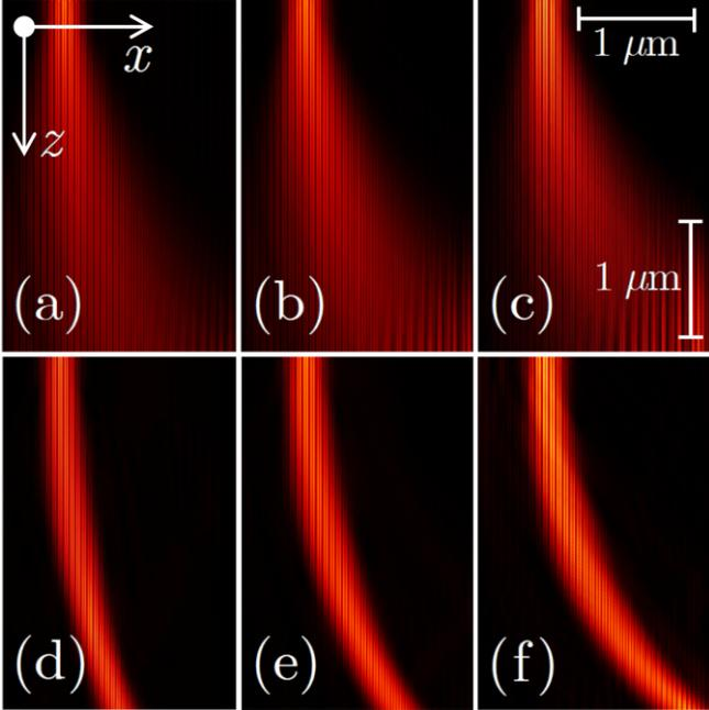
Fig. 2. Evolution dynamics in chirped subwavelength waveguide arrays in the linear (a)-(c) and nonlinear (d)-(f) regimes, in the absence of metallic losses. The chirp rate is  $\delta d = 0.5 \text{ nm}$  (a),(d),  $0.6 \text{ nm}$  (b),(e), and  $0.7 \text{ nm}$  in (c),(f). The propagation distance is  $3 \mu\text{m}$ , while the width of the transverse window is  $2 \mu\text{m}$ .
