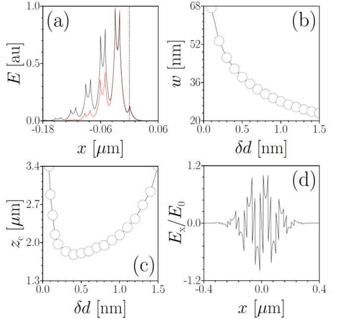
Fig. 5. (a) Profiles of stationary surface modes for  $\delta d = 0.4 \text{ nm}$  (black curve) and  $\delta d = 1.2 \text{ nm}$  (red curve). (b) Surface wave width versus  $\delta d$ . (c) Distance of the first collision with the interface for a beam initially centered at the 25<sup>th</sup> metallic layer, versus  $\delta d$ . (d) Input used for the excitation of self-deflecting solitons in the bulk of array at  $\delta d = 0.6 \text{ nm}$ .
