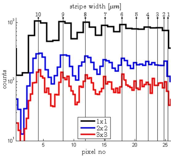
**Fig. 5** Pixel intensity profiles along one sub-pixel row indicated in Fig. 4 with red rims. The profiles are plotted for normal resolution (black line),  $2 \times 2$  (blue line), and  $3 \times 3$  (red line) sub-pixel division. Estimated positions of the Au bar centers are indicated with black vertical lines. On top the actual Au stripe widths are given.
