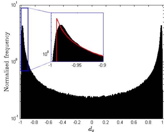
**Fig. 1** An example intensity ratio histogram of Au L photons generated from a real measurement (Au bar pattern) with formula (6). The histogram is normalized to occupy a unitary area and can be identified with the probability density function. In the inset the histogram is compared to Gaussian simulation (red line).
