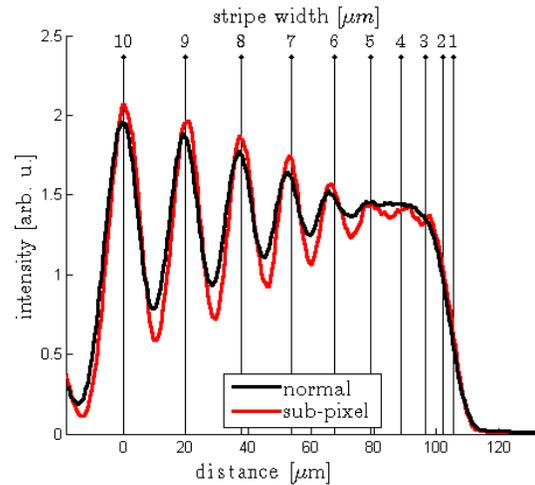
**Fig. 6** Intensity profile across Au bar structures calculated for normal resolution (black line) and  $3 \times 3$  sub-pixel division (red line) images. Estimated positions of the Au bar centers are indicated with black vertical lines. The intensity profile was constructed from data sampled at regular intervals across the Au bars. To increase the signal to noise ratio the intensity was integrated over the whole length of Au bars.
