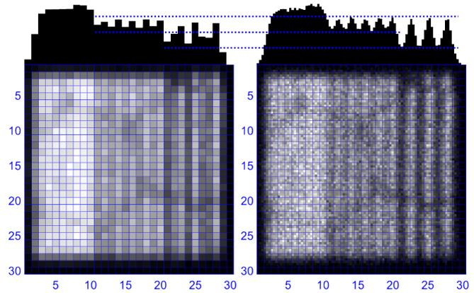
**Fig. 7** Normal resolution (left) and  $3 \times 3$  sub-pixel resolution (right) images of the Cu stripes pattern. The image was acquired at HS-PXBE beam line at HZDR with a parallel 1:1 optics. The grid shows the positions of the real pixels, each corresponding to  $48 \times 48 \mu\text{m}^2$  area on the sample surface. On top the cumulative intensity along each (sub-)pixel column is presented. The dotted guide lines indicate the contrast levels for the sub-pixel resolution image.
