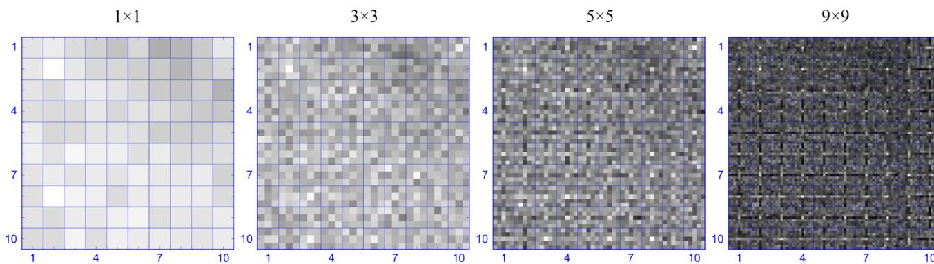
**Fig. 8** Normal resolution and  $3\times 3$ ,  $5\times 5$ , and  $9\times 9$  sub-pixel division images of a Au layer. The image was acquired at the BAMline at BESSY II with a 8:1 magnification lens. Artificial intensity structure following the pixel center position is strongly indicated for the sub-pixel resolution image. The grid shows the real pixel positions.
