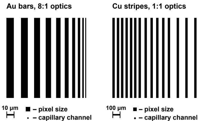
**Fig. 3** Sketch of Au bar pattern (left) and Cu stripes (right). Structures were measured with, respectively, focusing 8:1 and parallel 1:1 optics; sizes of corresponding pixels (side length of, respectively,  $6 \mu\text{m}$  and  $48 \mu\text{m}$ ) and capillary channels (entrance diameter of, respectively,  $2 \mu\text{m}$  and  $24 \mu\text{m}$ ) are shown for comparison.
