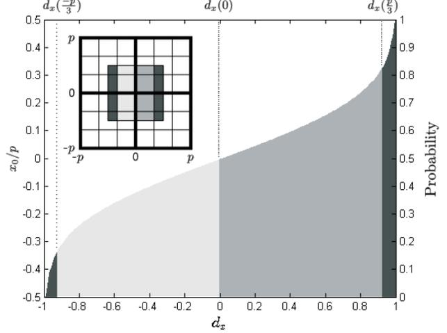
**Fig. 2** Relative photon hit position  $x_0$  calculated as a function of intensity ratio  $d_x$  according to equation (13). Likewise in Fig. 1 the data for Au L photons from Au bar pattern are illustrated. Secondary vertical axis shows cumulative probability distribution  $P_{d_x}$ . In the inset a  $2 \times 2$  pixel box with  $3 \times 3$  sub-pixel division is shown. Different levels of gray mark – in order from darkest to brightest – central, left and right sub-pixels.
