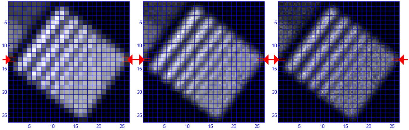
**Fig. 4** Normal resolution (left),  $2 \times 2$  (center) and  $3 \times 3$  (right) sub-pixel division images of the Au bar pattern. The image was acquired at the BAMline at BESSY II with an 8:1 magnification lens. The grid shows the positions of the real pixels, each corresponding to  $6 \times 6 \mu\text{m}^2$  area on the sample surface. Red flashes indicate the (sub-)pixel row chosen for comparison in Fig. 5.
