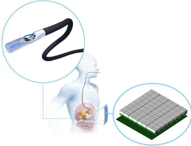
Figure 1: The EndoTOPPET-US detector with a magnification of the pancreatic endoscope (top circle) and the external plate (bottom circle).
