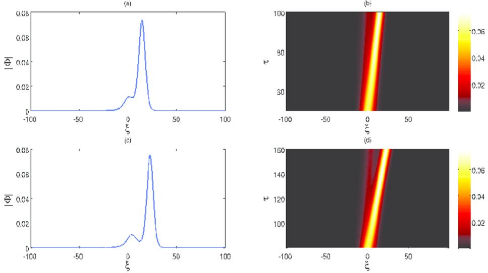
FIG. 2. The space-time evolution of the soliton profile  $|\Phi|$  [numerical solution of Eq. (30)] is shown at  $\tau = 100$  [Subplots (a) and (b)] and  $\tau = 160$  [Subplots (c) and (d)]. While the plots (a) and (c) show the soliton profiles with space, plots (b) and (d) are the corresponding contour plots. The parameter values are the same as for the dashed line in Fig. 1(d) and  $\sigma \sim 1$ .
