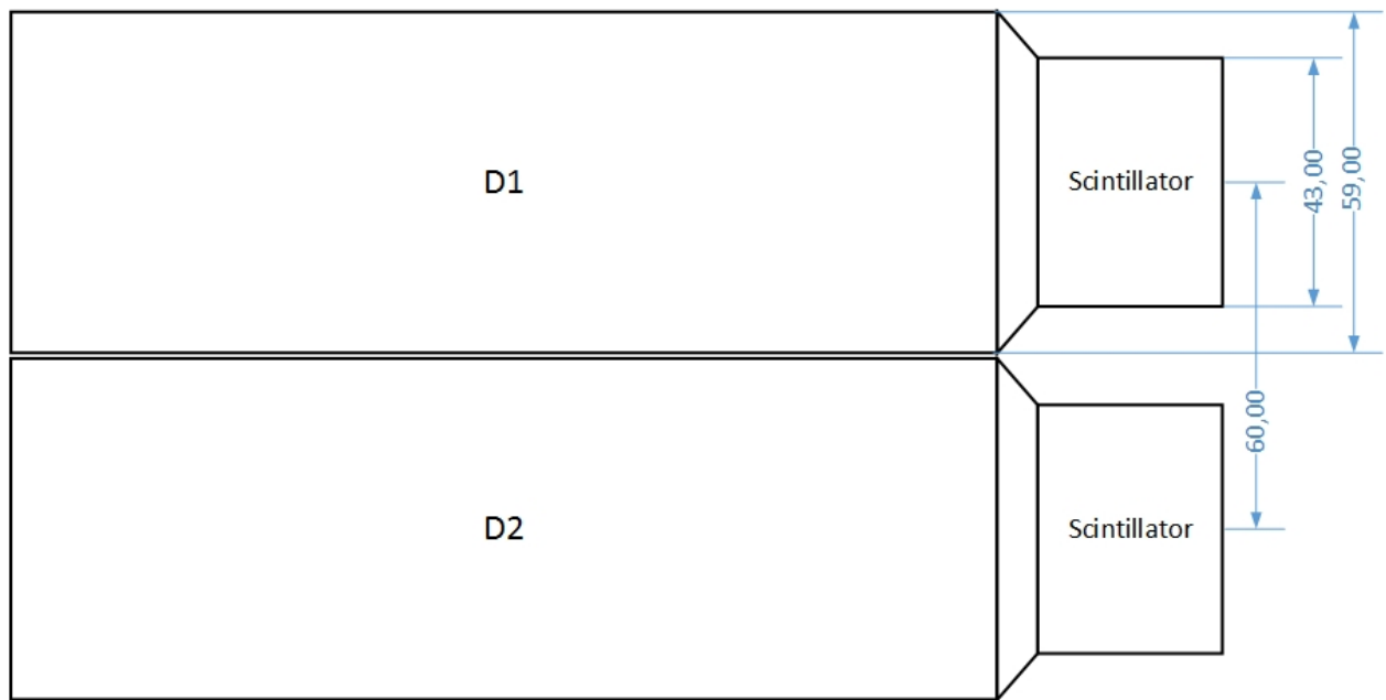
Figure 5. How the two cylindrical LaBr 3 scintillation detectors are placed next to each other. The detectors register an X-ray signal simultaneously during some discharges. This proves that the photon flux is high enough to cause a multiphoton registration at one detector.
