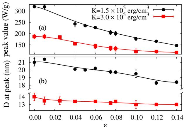
FIG. 5. Maximum SAR value (a) and peak position (b) as function packing fraction,  $\epsilon$  for two values of anisotropy:  $3 \times 10^5$  erg/cm<sup>3</sup> (red squares) and  $1.5 \times 10^5$  erg/cm<sup>3</sup> (black circles). The lines are to guide the eye.
