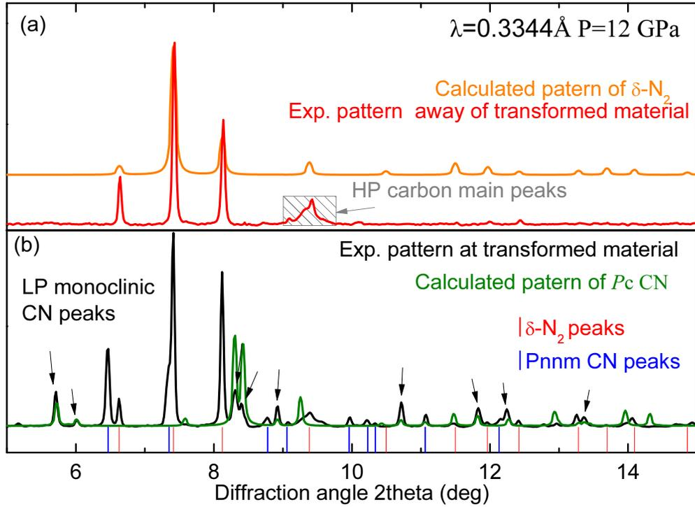
FIG. 6. X-ray diffraction pattern at 12 GPa: (a) Away from the synthesized material, the calculated pattern for  $\delta$  phase of  $\text{N}_2$  is plotted for clarity, (b) at the synthesized material, the calculated pattern for the LP CN monoclinic  $Pc$  phase is plotted with green. The experimental and theoretical (in brackets) lattice parameters are:  $a= 4.607(4.5421)\text{\AA}$ ,  $b= 3.172(3.2461)\text{\AA}$ ,  $c= 3.615(3.5429)\text{\AA}$ , and  $\beta= 110.85(108.855)\text{deg}$ .
