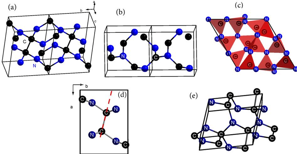
FIG. 1. **Schematic representations of:** (a)  $\beta$ -InS-type crystal structure of CN, (b) cg-CN, (c)  $\alpha$ - $\text{Si}_3\text{N}_4$ -type crystal structure of  $\text{C}_3\text{N}_4$ , (d) low and high pressure  $\beta$ -InS-type crystal structure of CN viewed along c-axis, the tilting of the C-C bond in respect to the a axis is highlighted by the red dashed line and (e) monoclinic  $Pc$  crystal structure of CN. Black and blue spheres indicate carbon and nitrogen atoms respectively.
