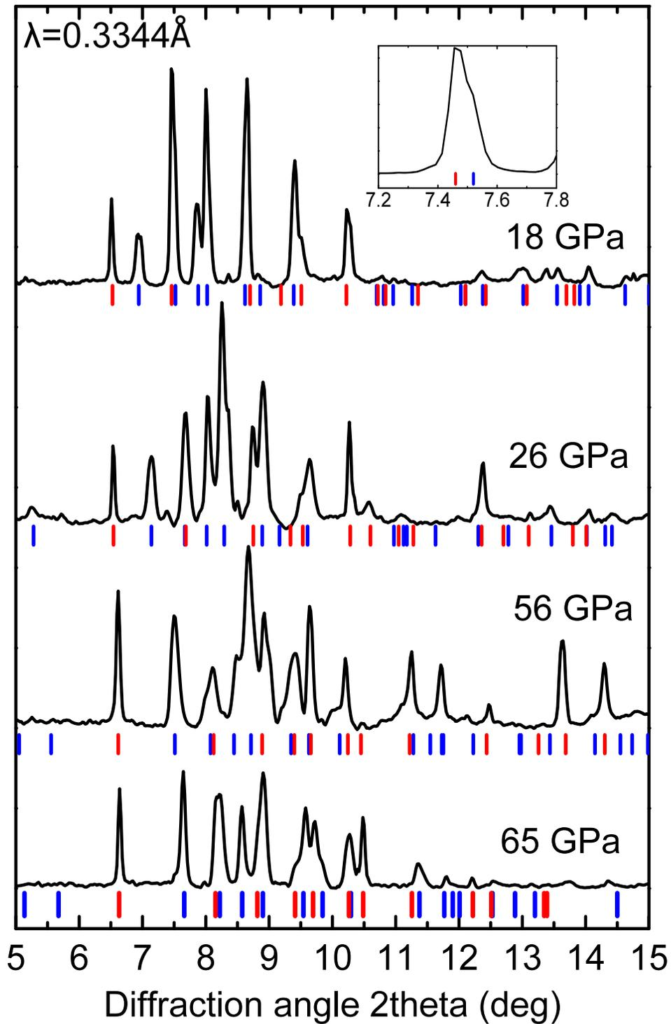
FIG. 5. X-ray diffraction patterns of CN at various pressures on pressure release after synthesis at 65 GPa. Expected positions of Bragg peaks of nitrogen and  $Pnnm$  CN phase are indicated with vertical blue and red ticks respectively.
