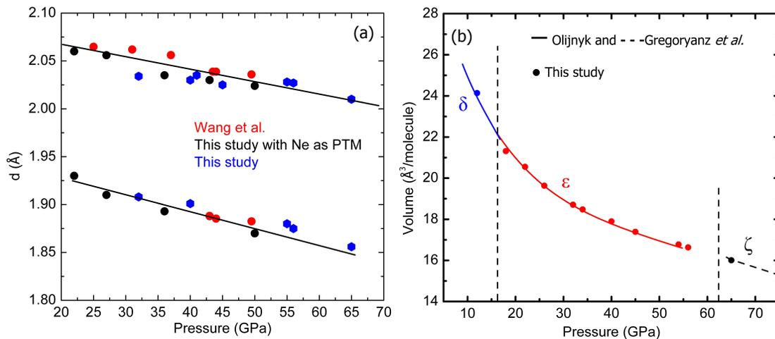
FIG. 3. (a) **d-spacing of the main peaks of the high pressure phase of carbon as a function of pressure:** Red symbols: Ref. [26] (starting from pure graphite with increasing pressure), Black symbols: this study (Ne as PTM) and Blue symbols: this study on pressure release. (b) **EOS of  $N_2$** , solid lines from Refs. [23,24], solid circles this study.
