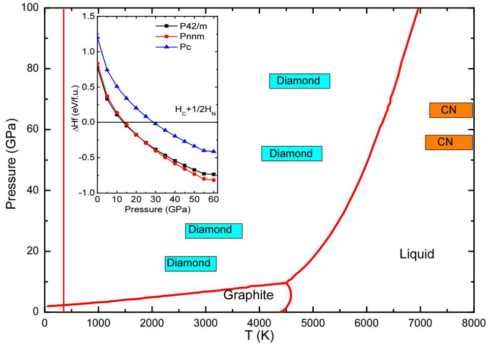
FIG. 1. Pressure-temperature phase diagram of carbon according to Ref. [27] together with pressure-temperature conditions (rectangles) of synthesis of *Pnnm* CN compound. The products as determined by XRD measurements are noted inside the rectangles. The inset shows the formation enthalpies per formula unit, determined by theoretical calculations of this study, of the tetragonal *P42/m*, orthorhombic *Pnnm* and monoclinic *Pc* CN phases relative to carbon and nitrogen as a function of pressure.
