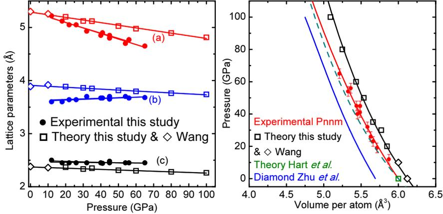
FIG. 4. Pressure dependence of (a) lattice parameters and (b) Volume per atom of *Pnnm* CN. Experimental data are shown with solid symbols and theoretical predictions with open ones. The solid curves in (b) are the third-order Birch EOS for diamond (blue) according to Zhu *et al.* [32], the synthesized CN phase (red) and theoretical EOS predicted for *Pnnm* CN (black) according to this study and Wang [18] and according to Hart *et al.* [15] (green).
