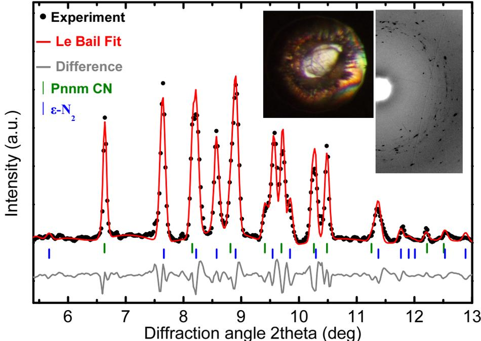
FIG. 2. **Le Bail refinement for CN at 65 GPa.** *Pnnm* CN and  $\zeta$ -N<sub>2</sub> peaks are marked with black and red vertical lines respectively. The X-ray wavelength is 0.3344 Å. The insets show: (a) a microphotograph of the sample after heating in transmitted light, indicating the transparency of the synthesized phase and (b) 2-D XRD image of the *Pnnm* CN and  $\zeta$ -N<sub>2</sub> mixture.
