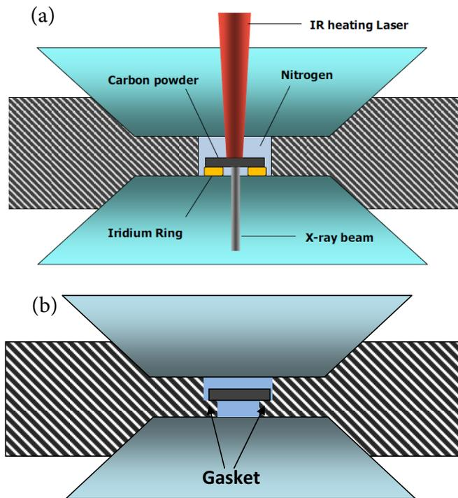
FIG. 7. Schematic representation of the cross-section of the experimental arrangements: a) Iridium ring spacer and b) recessed gasket. Double-sided LH has been performed but the schematic is simplified for clarity.
