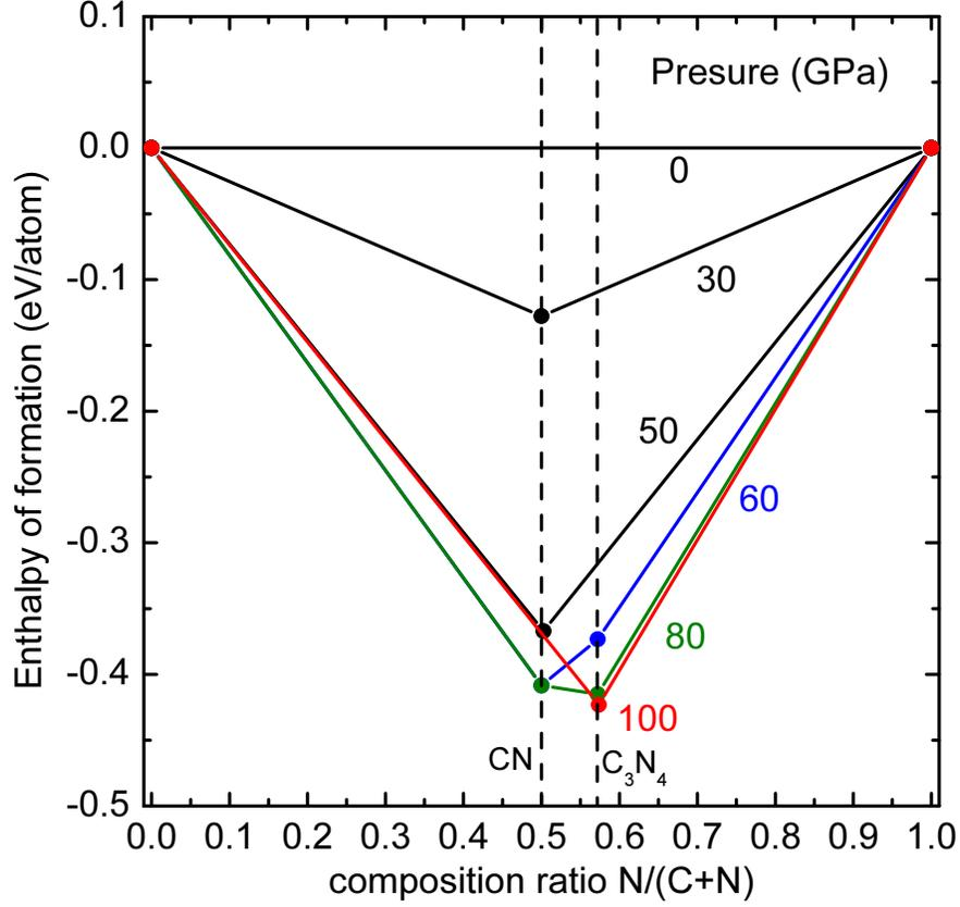
FIG. 2. Predicted convex hull diagrams of C-N system at selected pressures. Solid circles represent stable compounds.
