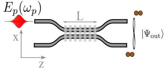
FIG. 1. Our source consists of a waveguide coupler, where the coupling region of length  $L$  is periodically poled. We couple ultrafast pump light into one waveguide of the fan-in region, where it propagates along the  $z$ -axis. After the periodically poled area, we use the fan-out region to separate the two output ports for our spatially entangled 2-photon N00N state  $|\Psi_{\text{out}}\rangle$ .
