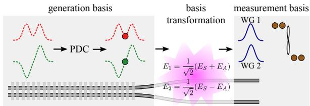
FIG. 3. At the beginning of the periodically poled coupler structure, the eigenmodes are unoccupied. During the PDC process, we generate photons with a certain probability only in the combination of symmetric and antisymmetric eigenmode. During the basis transformation a Hong-Ou-Mandel type interference takes place and cancels the coincidences between the two waveguide outputs, leading to the creation of post-processing free 2-photon N00N states.
