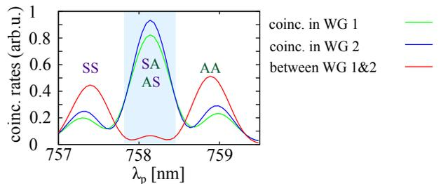
FIG. 4. The phase-matching scan by tuning the pump wavelength shows a clear suppression of coincidences between the two waveguide ports (red) in the middle of the phase-matching, while coincidences in the single waveguides peak (green: pumped waveguide, blue: unpumped waveguide).
