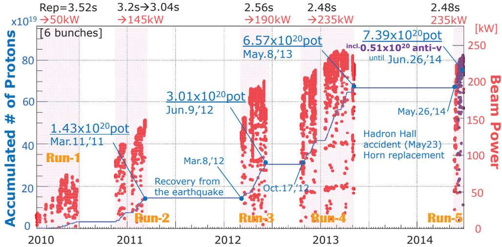
**Fig. 3.** Beam-power history (red dots plotted for each beam pulse) and accumulated numbers of protons-on-target (solid blue line) at the neutrino facility.
