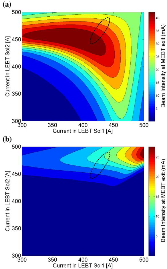
Figure 3: Simulated beam intensity at the MEBT exit as a function of the LEBT solenoid currents for a uniform neutralization factor along the LEBT of (a) 100% and (b) 60%. From TRACK. The ellipse mimics the measured area of favorable transmission reported in Fig. 2.
