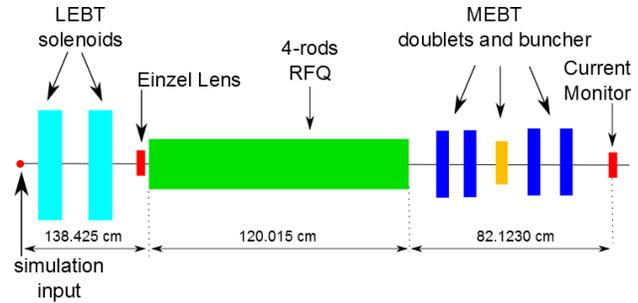
Figure 1: Layout of the FNAL Linac Injector.
